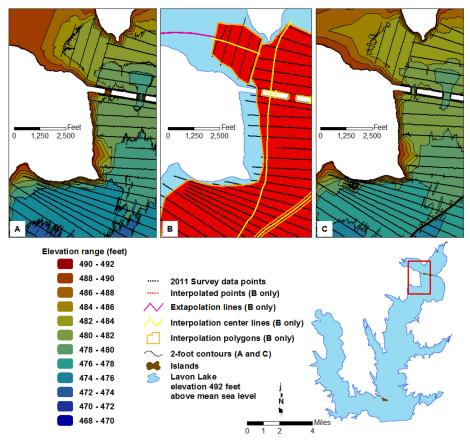
Figure 6. Anisotropic spatial interpolation and line extrapolation of Lavon Lake sounding data – A) bathymetric contours without interpolated points, B) sounding points (black) and interpolated points (red), C) bathymetric contours with the interpolated points
