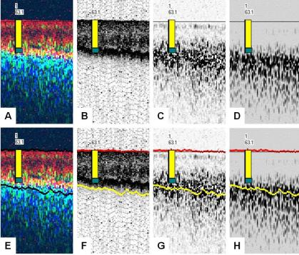
Figure 8. Comparison of sediment core L-1 with acoustic signal returns A,E) combined acoustic signal returns, B,F) 200 kHz frequency, C,G) 50 kHz frequency, D,H) 24 kHz frequency
