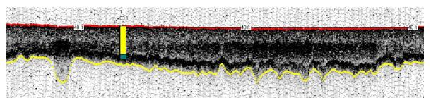
Figure 9. Cross-section of data collected during 2011 survey, displayed in DepthPic (200 kHz frequency), correlated with sediment core sample L-1 and showing the current surface in red and pre-impoundment surface in yellow
