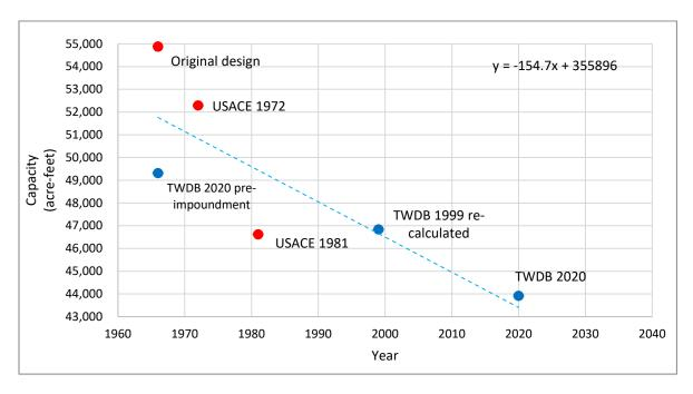
Figure 10. Plot of current and previous capacity estimates (acre-feet) at elevation 421.00 feet. Capacity estimates for each TWDB survey plotted as blue dots and other surveys as red dots. The blue trend line illustrates the total average loss of capacity through 2020.
