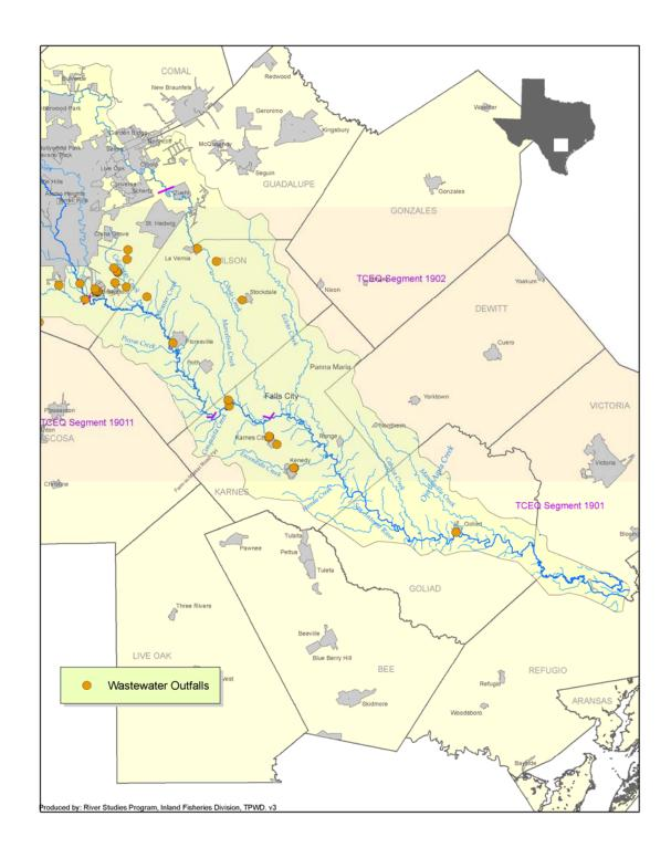
**Figure 6.** Wastewater discharge locations on the lower San Antonio River and Cibolo Creek.
