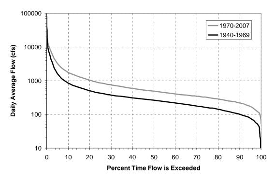
**Figure 3.** Flow duration curves for daily average flow at USGS gage 08188500, San Antonio River at Goliad.
