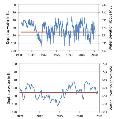
The late September water-level measurement in this Edwards (Balcones Fault Zone) Aquifer well, elevation 731 feet above mean sea level, was 67.40 feet below land surface, or 663.60 feet above mean sea level. This was 7.50 feet above last month's measurement, 2.90 feet below last year's measurement and 20.76 feet below the initial measurement recorded in 1932.
