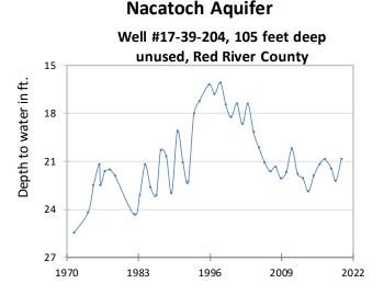
The initial water-level measurement taken by the TWDB in this well was in April of 1971 at 25.48 feet below land surface. The TWDB has collected a water-level measurement in this well nearly every year since. The period of record reveals a gradual increase of just over 4.6 feet in 48 years with the highest water level of 16.2 feet below land surface measured in November of 1995.
