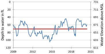
The water-level late May in this **Edwards** measurement (Balcones Fault Zone) Aquifer well, elevation 731 feet above mean sea level, was 59.40 feet below land surface, or 671.60 feet above mean sea level. This was 5.10 feet above last month's measurement, 8.40 feet below last year's measurement and 12.76 feet below the initial measurement recorded in 1932.
