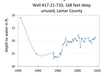
The initial measurement of 11 feet below land surface was recorded by a registered water well driller in August of 1942. Roughly thirty-three years later, the TWDB began recording near-annual measurements in the public supply well. The period of record reveals a sharp decline in water level over the first sixteen years of well use. After 1958, water levels increased and have remained around 19 feet below land surface. This is likely a result of the well no longer being used.
