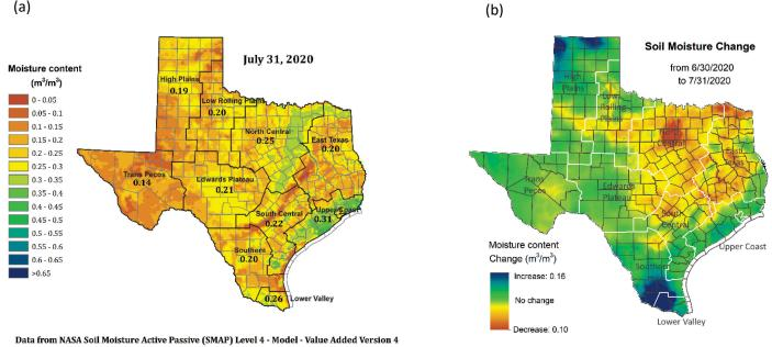
Soil moisture content is shown as volume of water per unit volume of bulk soil. Root zone: 0 to 1 meter depth.
