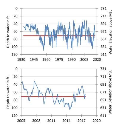
The late September water-level measurement in this Edwards (Balcones Fault Zone) Aquifer well, elevation 731 feet above mean sea level, was 66.21 feet below land surface, or 664.79 feet above mean sea level. This was 0.40 feet below last month's measurement, 13.50 feet below last year's measurement, and 19.57 feet below the initial measurement recorded in 1932.
