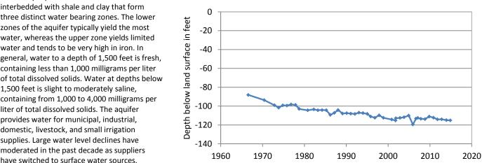
The water level in this domestic and livestock well has gradually yet steadily declined from the initial measurement of 88.15 feet below land surface in 1966. The TWDB has been measuring this well since 1970. The lowest measurement was observed at 119.5 feet below land surface in 2005.
