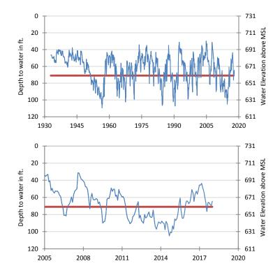
The late December water-level measurement in this Edwards (Balcones Fault Zone) Aquifer well, elevation 731 feet above mean sea level, was 64.41 feet below land surface, or 666.59 feet above mean sea level. This was 5.00 feet above last month's measurement, 18.90 feet below last year's measurement, and 17.77 feet below the initial measurement recorded in 1932.
