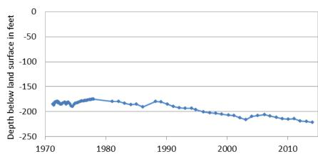
Drilled as an observation well by the TWDB in 1971, this well has 76 water level measurements to date. The water level remained relatively unchanged since1971, although a gradual decline has occurred since the early1990s.
