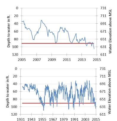
The late August water level measurement in this Edwards (BFZ) Aquifer well, elevation 731 feet above mean sea level, was 105 feet below land surface, or 626 feet above mean sea level. This was 7.8 feet below last month's measurement, 7.8 feet below last year's measurement, and 58.36 feet below the initial measurement recorded in 1932.
