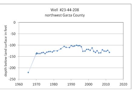
quality is poorer than the overlying Ogallala This unused irrigation well, at a total depth of 271 feet and elevation of 3,015 feet, Aquifer and in excess of 20,000 milligrams has been used as a water-level observation wells since 1970.
