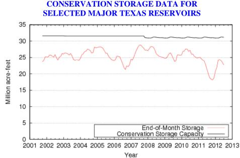
Figures are based on the end of the month data at 109 major reservoirs that represent 96 percent of the total conservation storage capacity of the 175 major water supply reservoirs in Texas. Major reservoirs are defined as having a conservation storage capacity of 5,000 acre-feet or greater.
