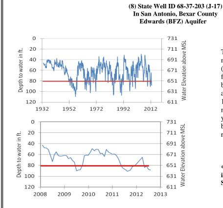
The late July water level measurement in this Edwards (BFZ) Aquifer well, elevation 731 feet above sea level, was 88.47 feet below land surface, or 642.53 feet above mean sea level. This was 1.11 feet below last month's measurement, 0.41 feet below last year's measurement, and 41.83 feet below the initial measurement recorded in 1932.
