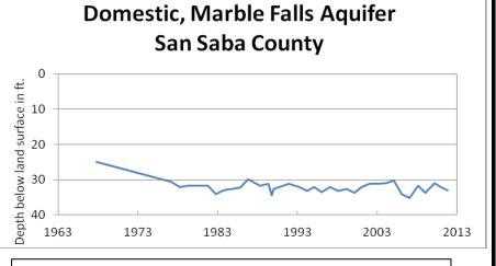
Water levels in this domestic well, at an elevation of 1,100 feet above sea level in eastern San Saba County, experienced a total historical decline of eight feet from the original measurement in 1967 until the latest measurement in 2011, with levels remaining relatively constant since the late seventies. TEXAS WATER DEVELOPMENT BOARD 1700 N. CONGRESS AVE. P.O. BOX 13231 AUSTIN TX 78711-3231
