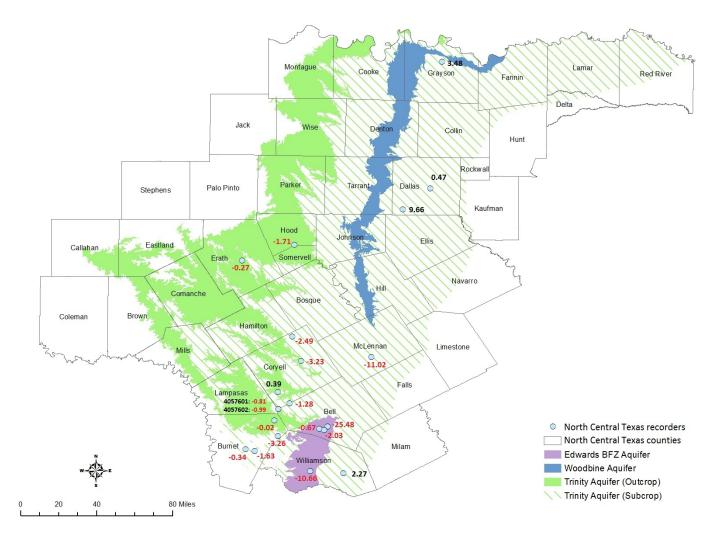
**Figure 5-1**. Location of wells with TWDB-operated automatic water-level recorders in northern Central Texas. Water-level changes from 2013 to 2014 are shown in feet. Black indicates a rise in water levels, and red indicates decline. BFZ = Balcones Fault Zone.
