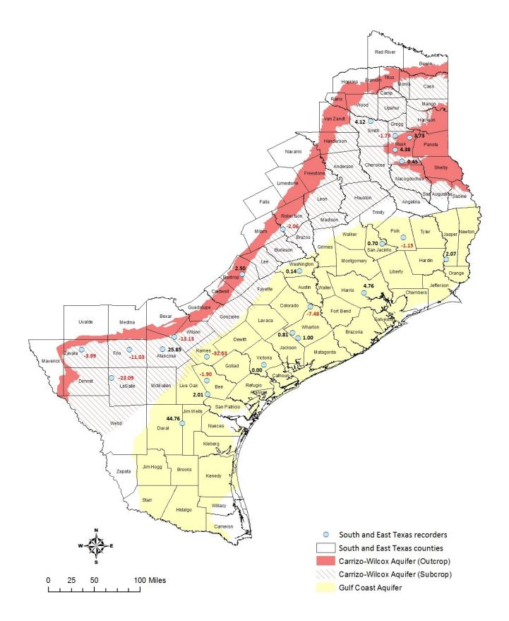
**Figure 6-1**. Location of wells with TWDB-operated automatic water-level recorders in South and East Texas. Water-level changes from 2012 to 2013 are shown in feet. Black indicates a rise in water levels, and red indicates decline.
