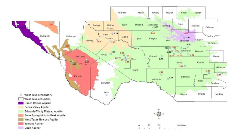
**Figure 4-1.** Location of wells with TWDB-operated automatic water-level recorders in West Texas. Water-level changes from 2013 to 2014 are shown in feet. Black indicates a rise in water levels, and red indicates decline.
