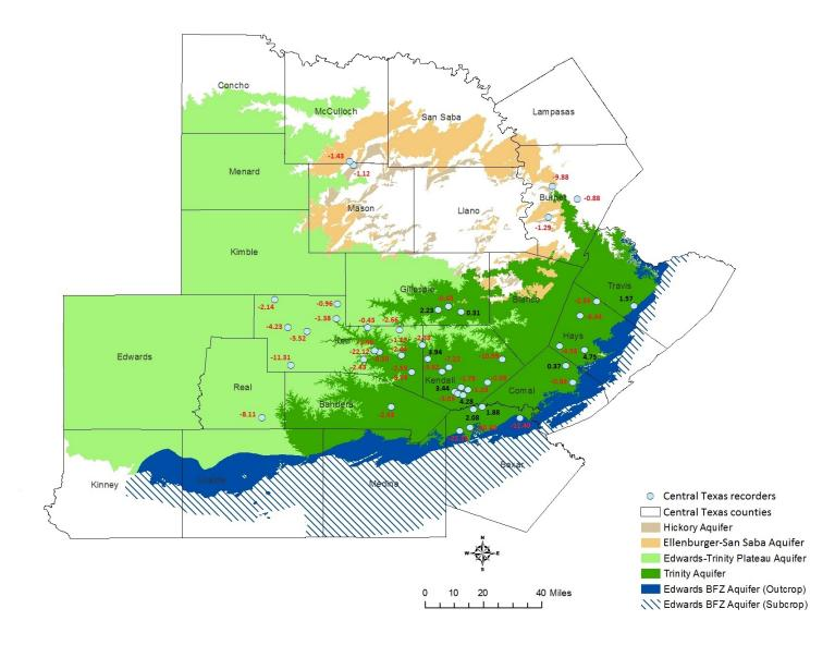
**Figure 7-1**. Location of wells with TWDB-operated automatic water-level recorders in Central Texas. Water-level changes from 2012 to 2013 are shown in feet. Black indicates a rise in water level and red indicates decline. BFZ = Balcones Fault Zone.
