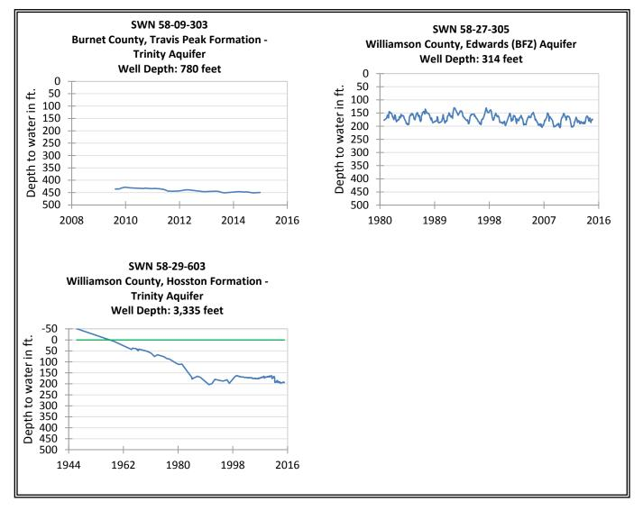
**Figure 5-2** (continued) Hydrographs of TWDB recorder wells in northern Central Texas. SWN = state well number, BFZ = Balcones Fault Zone
