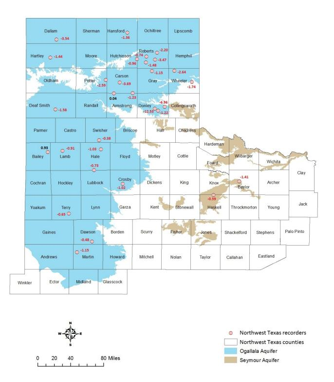
**Figure 3-1**. Location of wells with TWDB-operated automatic water-level recorders in Northwest Texas. Water-level changes from 2013 to 2014 are shown in feet. Black indicates a rise in water levels, and red indicates a decline.
