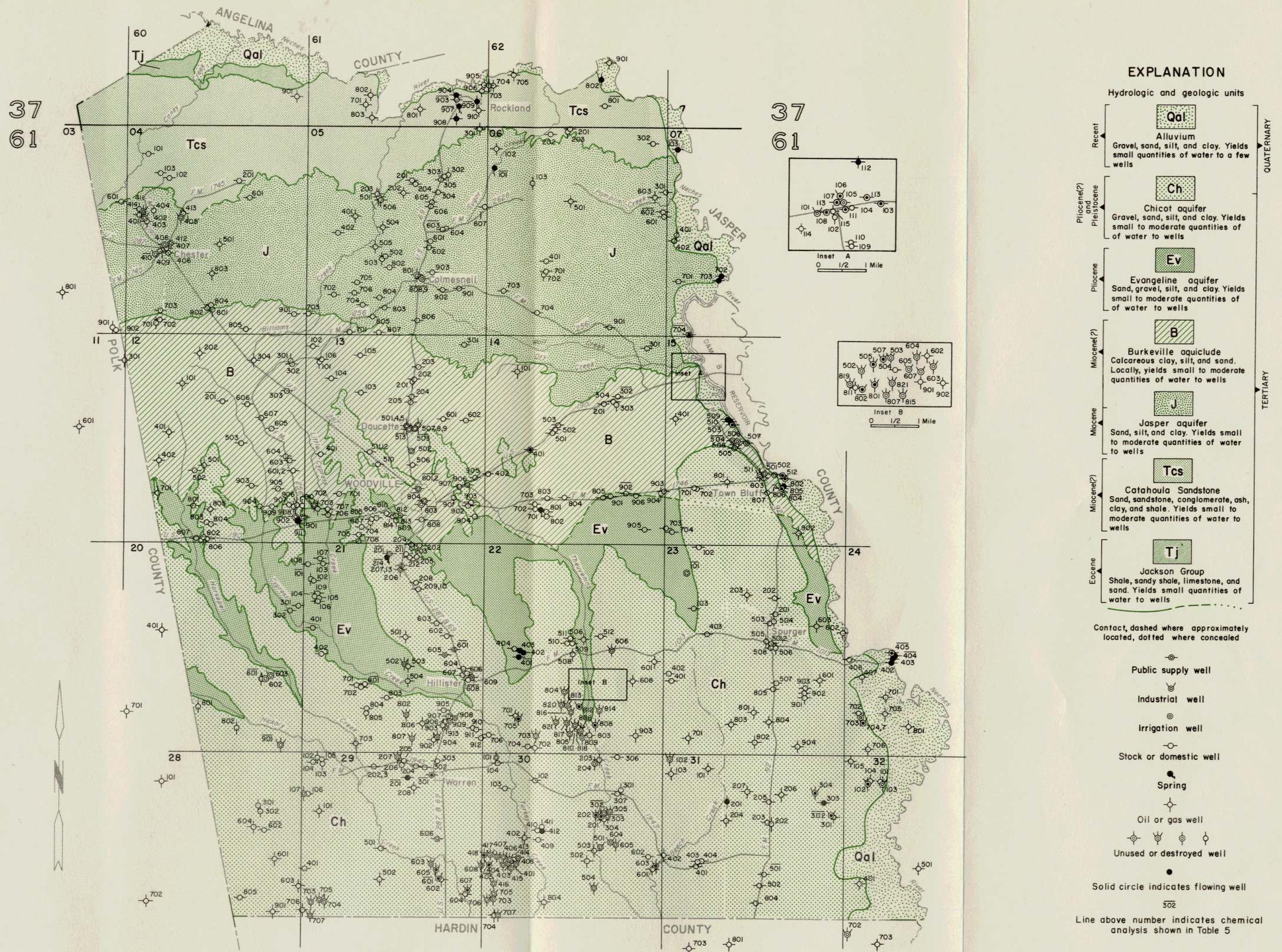
Figure 12 Hydrologic and Geologic Units and Locations of Wells and Springs in Tyler County and Adjacent Areas
