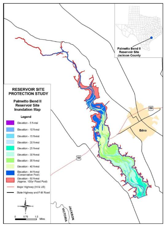
Figure 5-65. Inundation map for Palmetto Bend Reservoir—Stage II. ft-msl=feet above mean sea level
