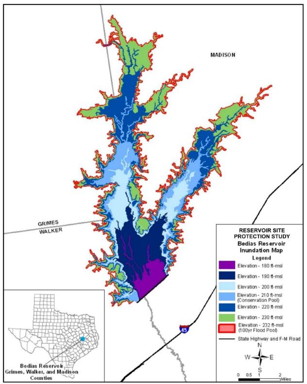
Figure 5-3. Inundation map for Bedias Reservoir. ft-msl=feet above mean sea level
