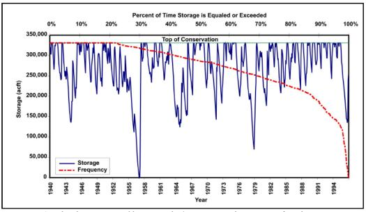
Figure 5-81. Simulated storage in Parkhouse II Lake (conservation elevation=410 feet; diversion=144,300 acre-feet per year).
