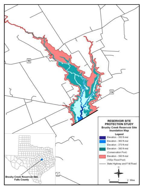
Figure 5-15. Inundation map for Brushy Creek Reservoir. ft-msl=feet above mean sea level
