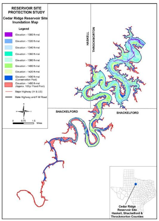
Figure 5-21. Inundation map for Cedar Ridge Reservoir. ft-msl=feet above mean sea level
