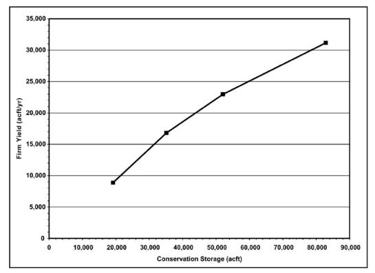
Figure 5-66. Firm yield versus conservation storage for Palmetto Bend Reservoir–Stage II. acft/yr=acre-feet per year
