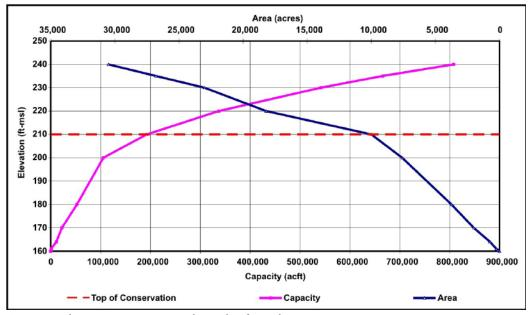
Figure 5-2. Elevation-area-capacity relationship for Bedias Reservoir. ft-msl=feet above mean sea level; acft=acre-feet
