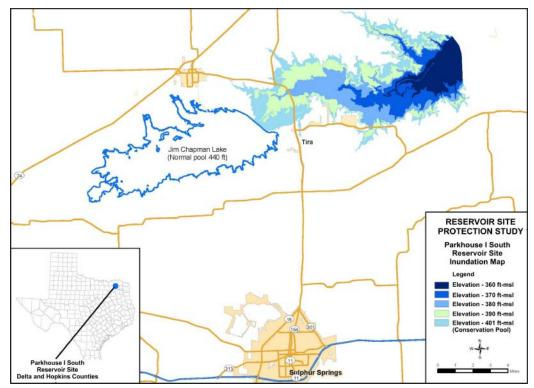
Figure 5-72. Inundation map for Parkhouse I Lake. ft-msl=feet above mean sea level
