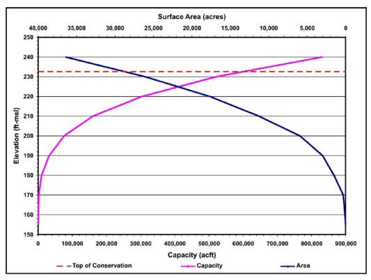
Figure 5-27. Elevation-area-capacity relationship for Cuero II Reservoir. ft-msl=feet above mean sea level; acft=acre-feet
