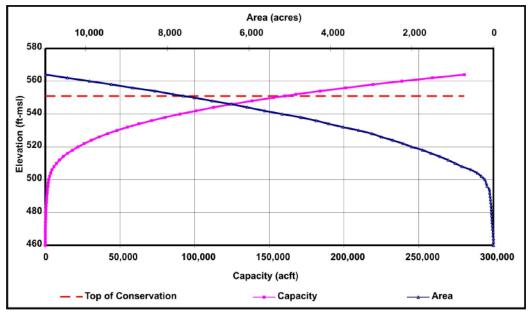
Figure 5-85. Elevation-area-capacity relationship for Lake Ralph Hall. ft-msl=feet above mean sea level; acft=acre-feet
