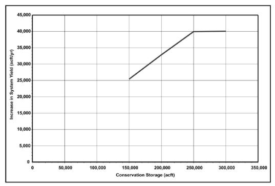
Figure 5-58. Firm yield versus conservation storage for the Nueces Off-Channel Reservoir. acft/yr=acre-feet per year
