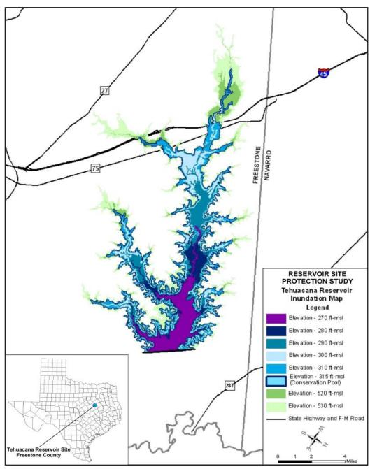
Figure 5-100. Inundation map for Tehuacana Reservoir. ft-msl=feet above mean sea level
