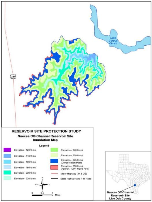
Figure 5-57. Inundation map for Nueces Off-Channel Reservoir. ft-msl=feet above mean sea leve
