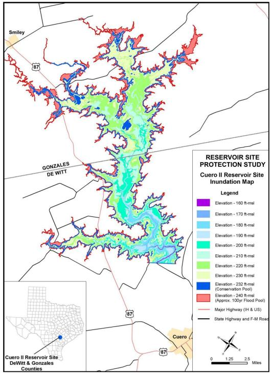
Figure 5-28. Inundation map for Cuero II Reservoir. ft-msl=feet above mean sea level
