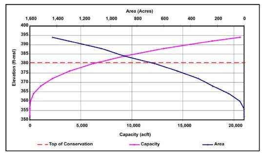
Figure 5-14. Elevation-area-capacity relationship for Brushy Creek Reservoir. ft-msl=feet above mean sea level; acft=acre-feet
