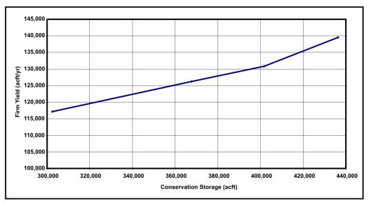
Figure 5-44. Firm yield versus conservation storage for Lower Bois d'Arc Creek Reservoir. acft/yr=acre-feet per year
