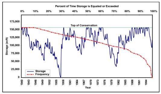
Figure 5-87. Simulated storage in Lake Ralph Hall (conservation elevation=551 feet; diversion=32,940 acre-feet per year).
