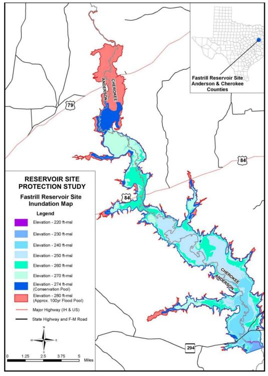
Figure 5-36. Inundation map for Fastrill Reservoir. ft-msl=feet above mean sea level
