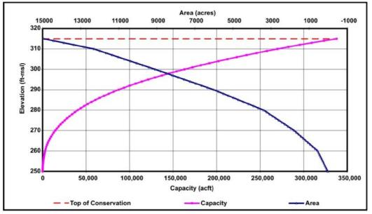
Figure 5-98. Elevation-area-capacity relationship for Tehuacana Reservoir. ft-msl=feet above mean sea level; acft=acre feet
