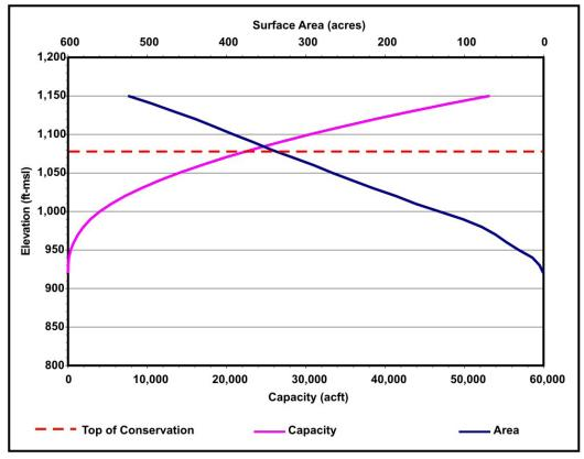
Figure 5-106. Elevation-area-capacity relationship for Wilson Hollow Reservoir. ft-msl=feet above mean sea level; acft=acre-feet
