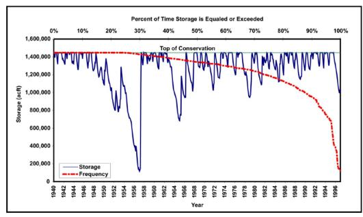
Figure 5-102. Simulated storage in Tehuacana and Richland-Chambers reservoirs (conservation elevation=315 feet; incremental yield=41,900 acre-feet per year). acft=acre-feet
