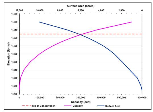
Figure 5-20. Elevation-area-capacity relationship for Cedar Ridge Reservoir. ft-msl=feet above mean sea level; acft=acre-feet
