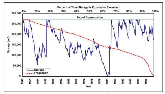
Figure 5-94. Simulated storage in Ringgold Reservoir (conservation elevation=844 feet; diversion=32,800 acre-feet per year). acft=acre-feet
