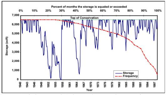
Figure 5-16. Simulated storage in Brushy Creek Reservoir (conservation elevation=380.5 feet; diversion=1,380 acre-feet per year).
