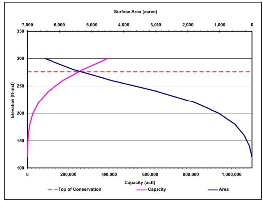
Figure 5-56. Elevation-area-capacity relationship for Nueces Off-Channel Reservoir. ft-msl=feet above mean sea level; acft=acre-feet
