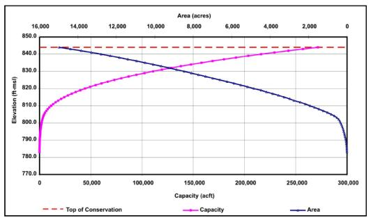
Figure 5-91. Elevation-area-capacity relationship for Ringgold Reservoir. ft-msl=feet above mean sea level; acft=acre feet
