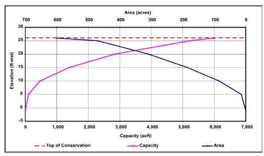
Figure 5-9. Elevation-area-capacity relationship for Brownsville Weir and Reservoir. ft-msl=feet above mean sea level; acft=acre-feet
