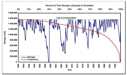
Figure 5-52. Simulated storage in Marvin Nichols IA Reservoir (conservation elevation=328 feet; diversion=602,000 acre-feet per year). acft=acre-feet per year
