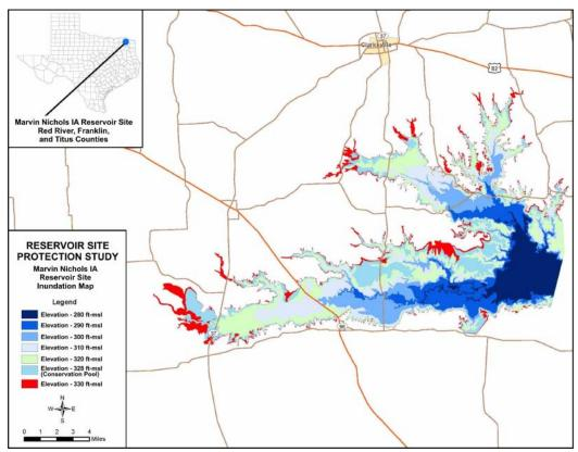
Figure 5-50. Inundation map for Marvin Nichols IA Reservoir. ft-msl=feet above mean sea level
