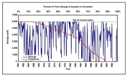
Figure 5-10. Simulated storage in Brownsville Weir and Reservoir (conservation elevation=26 feet; diversion=20,643 acre-feet per year). acft=acre-feet
