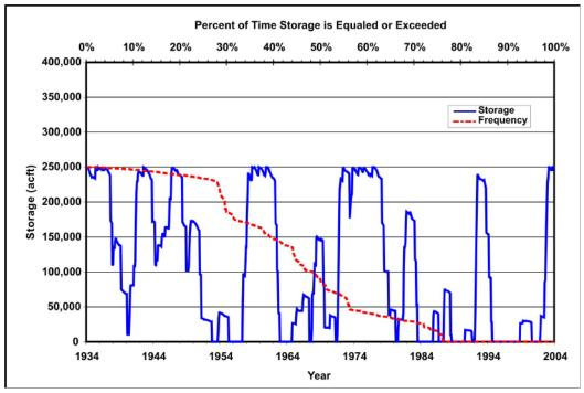
Figure 5-59. Simulated storage in the Nueces Off-Channel Reservoir (conservation elevation=275.3 feet; incremental yield=39,935 acre-feet per year). acft=acre-feet
