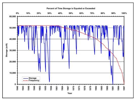
Figure 5-67. Simulated storage in Palmetto Bend Reservoir–Stage II (conservation elevation=44 feet; diversion=2,964 acre-feet per year).
