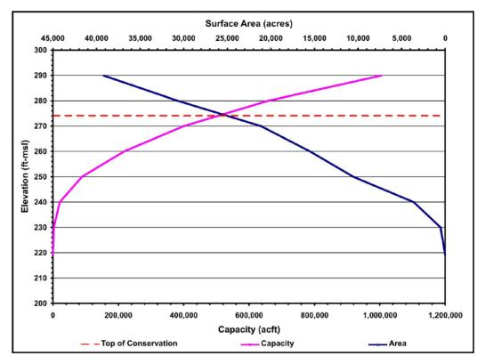
Figure 5-35. Elevation-area-capacity relationship for Fastrill Reservoir. ft-msl=feet above mean sea level; acft=acre-feet
