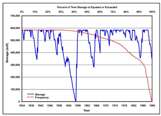
Figure 5-30. Simulated storage in Cuero II Reservoir (conservation elevation=232 feet; diversion=71,437 acre-feet per year). acre-feet
