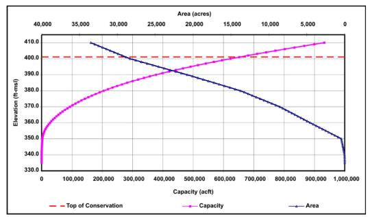
Figure 5-71. Elevation-area-capacity relationship for Parkhouse I Lake. ft-msl=feet above mean sea level; acft=acre-feet
