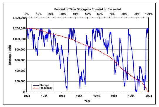
Figure 5-60. Simulated combined storage for Lake Corpus Christi, Choke Canyon Reservoir, and Nueces Off-Channel Reservoir (system diversion=271,860 acre-feet per year).
