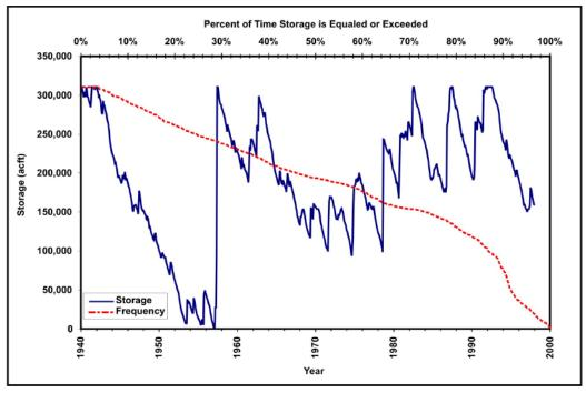
Figure 5-23. Simulated storage in Cedar Ridge Reservoir (conservation elevation=1,430 feet; diversion=36,891 acre-feet per year). acft=acre-feet
