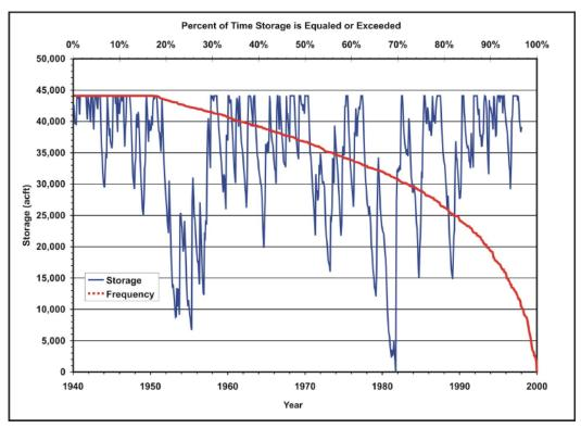
Figure 5-110. Simulated system storage for Lake Palo Pinto and Wilson Hollow reservoirs (system diversion=17,213 acre-feet per year). acft=acre-feet
