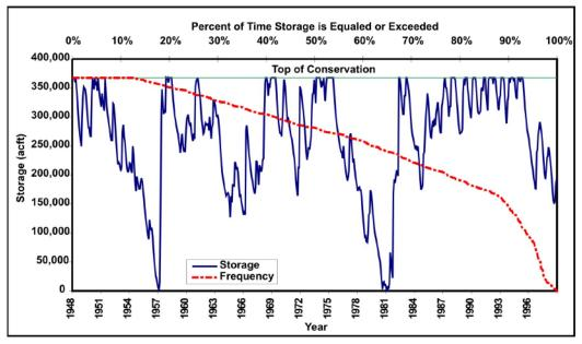
Figure 5-45. Simulated storage in Lower Bois d'Arc Creek Reservoir (conservation elevation=534 feet; diversion=126,280 acre-feet per year) acft=acre-feet
