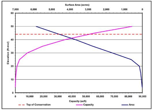
Figure 5-64. Elevation-area-capacity relationship for Palmetto Bend Reservoir–Stage II. ft-msl=feet above mean sea level; acft= acre-feet
