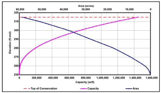
Figure 5-99. Elevation-area-capacity relationship for Tehuacana and Richland-Chambers reservoirs combined.
