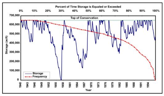
Figure 5-74. Simulated storage in Parkhouse I Lake (conservation elevation=401 feet; diversion= 22,000 acre-feet per year).
