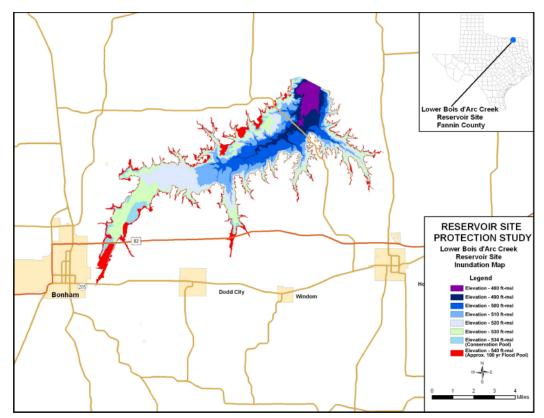
Figure 5-43. Inundation map for Lower Bois d'Arc Creek Reservoir. ft-msl=feet above mean sea level
