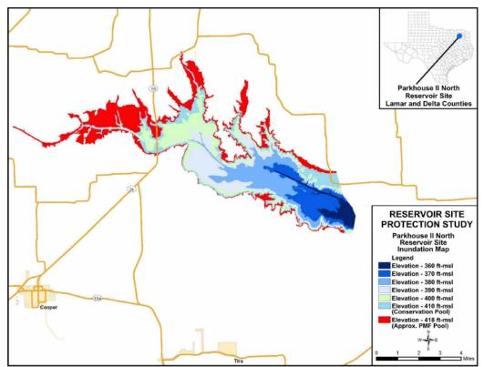
Figure 5-79. Inundation map for Parkhouse II Lake. ft-msl=feet above mean sea level; PMF=probable maximum flood
