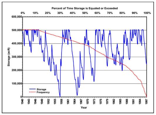
Figure 5-38. Simulated storage in Fastrill Reservoir (conservation elevation=274 feet; diversion=134,038 acre-feet per year).
