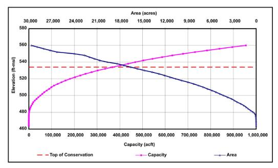
Figure 5-42. Elevation-area-capacity relationship for Lower Bois d'Arc Creek Reservoir. ft-msl=feet above mean sea level; acft=acre-feet
