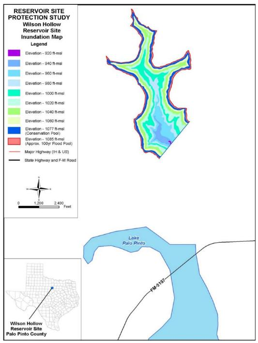
Figure 5-107. Inundation map for Wilson Hollow Reservoir. ft-msl=feet above mean sea level
