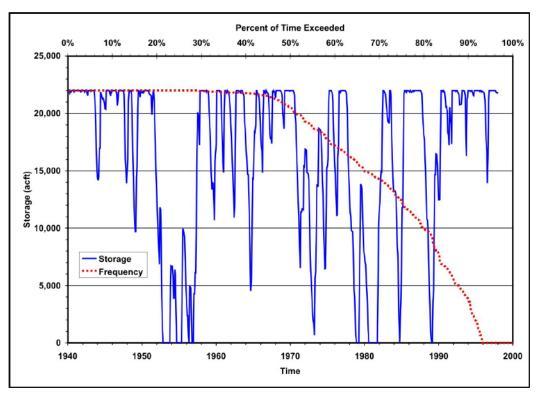
Figure 5-109. Simulated storage in Wilson Hollow Reservoir (conservation elevation=1,077 feet; incremental diversion=873 acre-feet per year). acft=acre-feet
