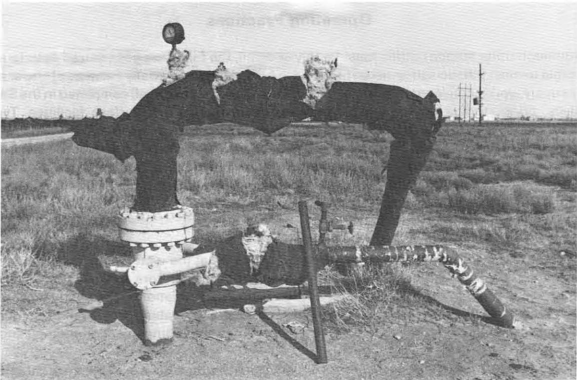
Figure 5-4.—Typical Brine Well
