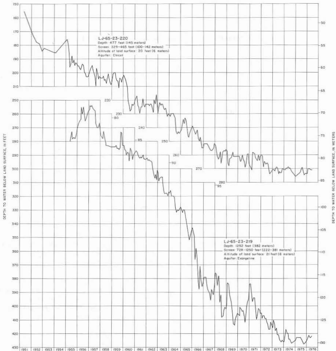
Figure 11.—Hydrographs Showing Changes in Water Levels in Wells in the Pasadena Area
