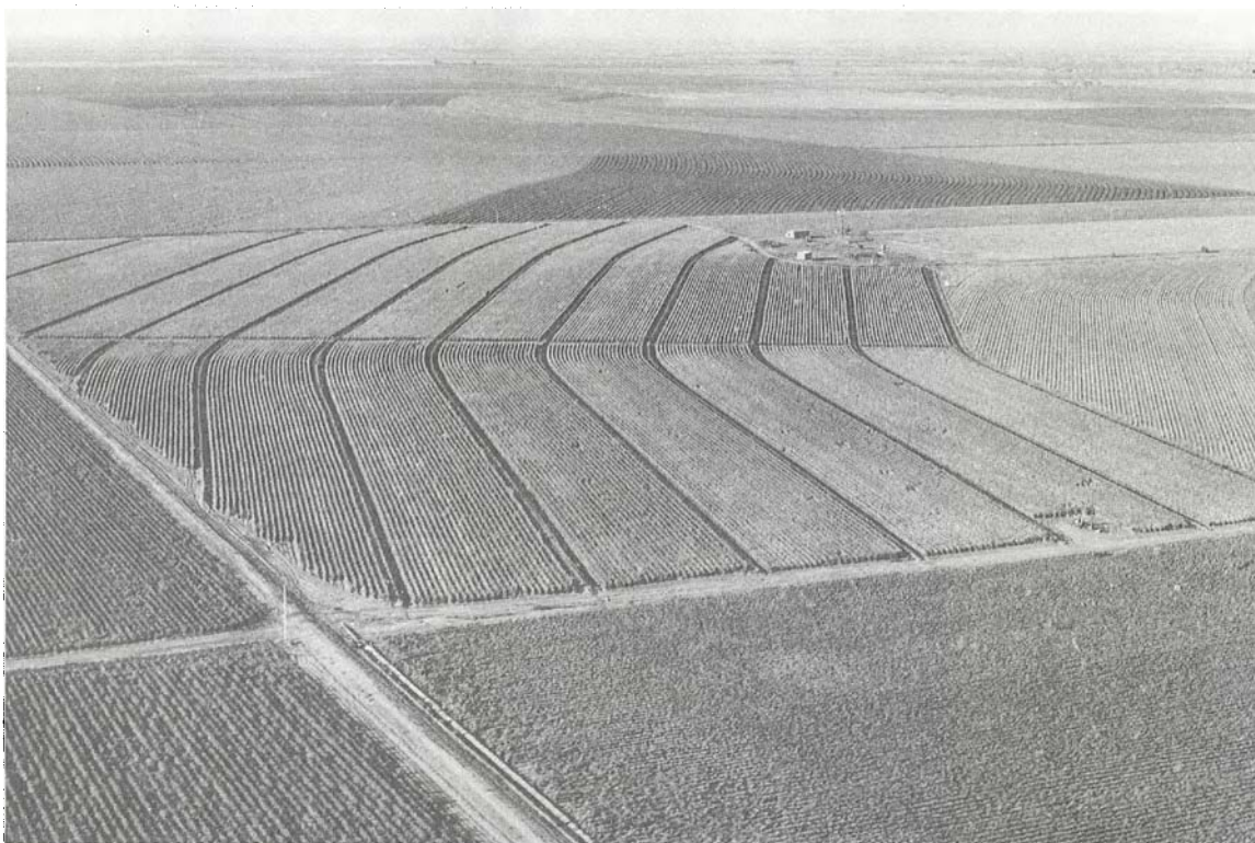
Bench leveling of cropland is a water-conservation practice that retards runoff and promotes infiltration. This view is near Crosbyton on the High Plains. Photo courtesy U.S. Soil Conservation Service.
