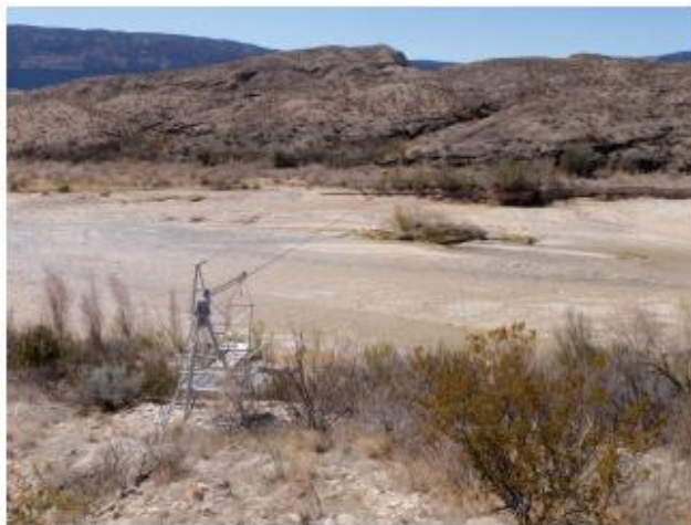
Figure 3.2-4. Photo of the Terlingua Creek gage and cableway. Photo is taken from left bank and flow is from right to left.
