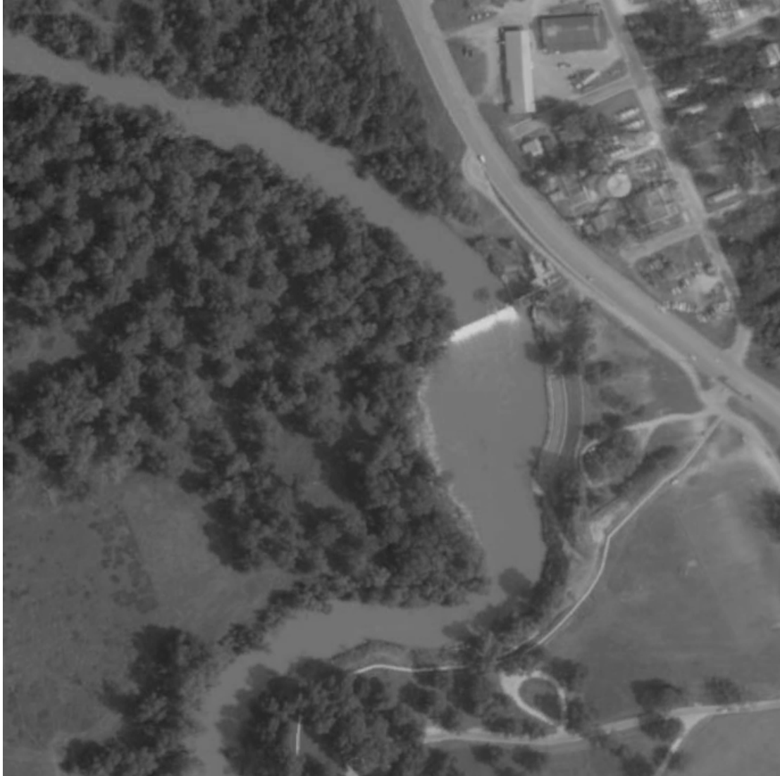
Figure 12. Widening below a run-of-river dam on the Guadalupe River at Gonzales. The channel upstream of the dam (top of photo) is 66 to 90 ft (20 to 27 m) wide, while the widened area downstream is up to 312 ft (95 m) wide.
