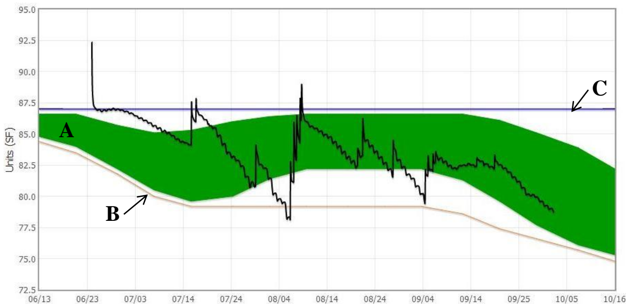
Figure 4: The summary graph for all sensors in an AquaSpy Probe. A) The green area is the optimal level for the soil moisture for the crop. B) The red line represents the refill point. C) The blue line represents the field capacity for the soil.
