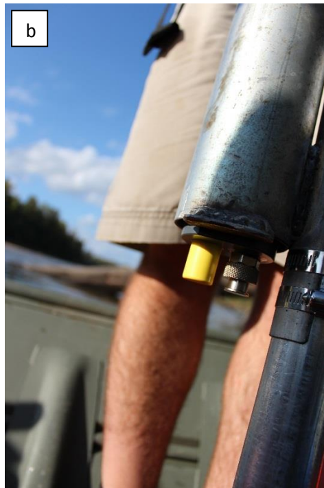
Figure 10. Submersible Ultrasonic Receiver (SUR) a) Getting locked into metal sleeve b) Hydrophone (yellow) rotated to point towards middle of Sabine River, October 2012.
