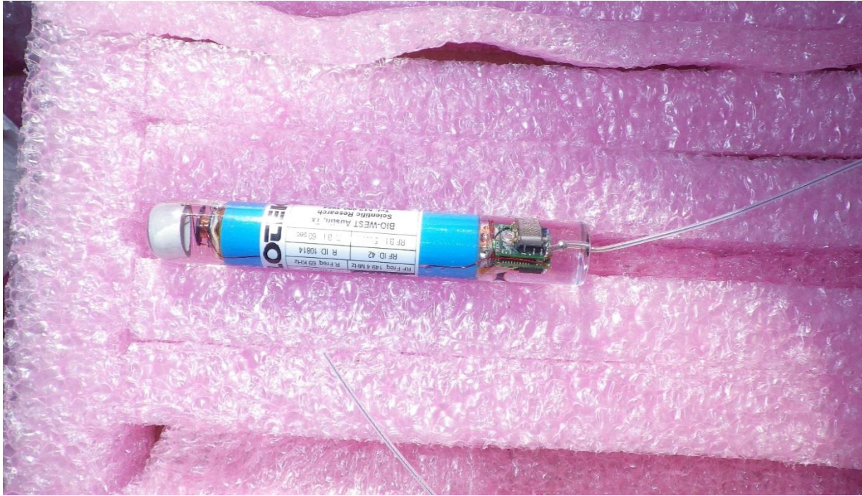
Figure 5. A Combined Acoustic / Radio Transmitters (CART) tag prior to implantation.
