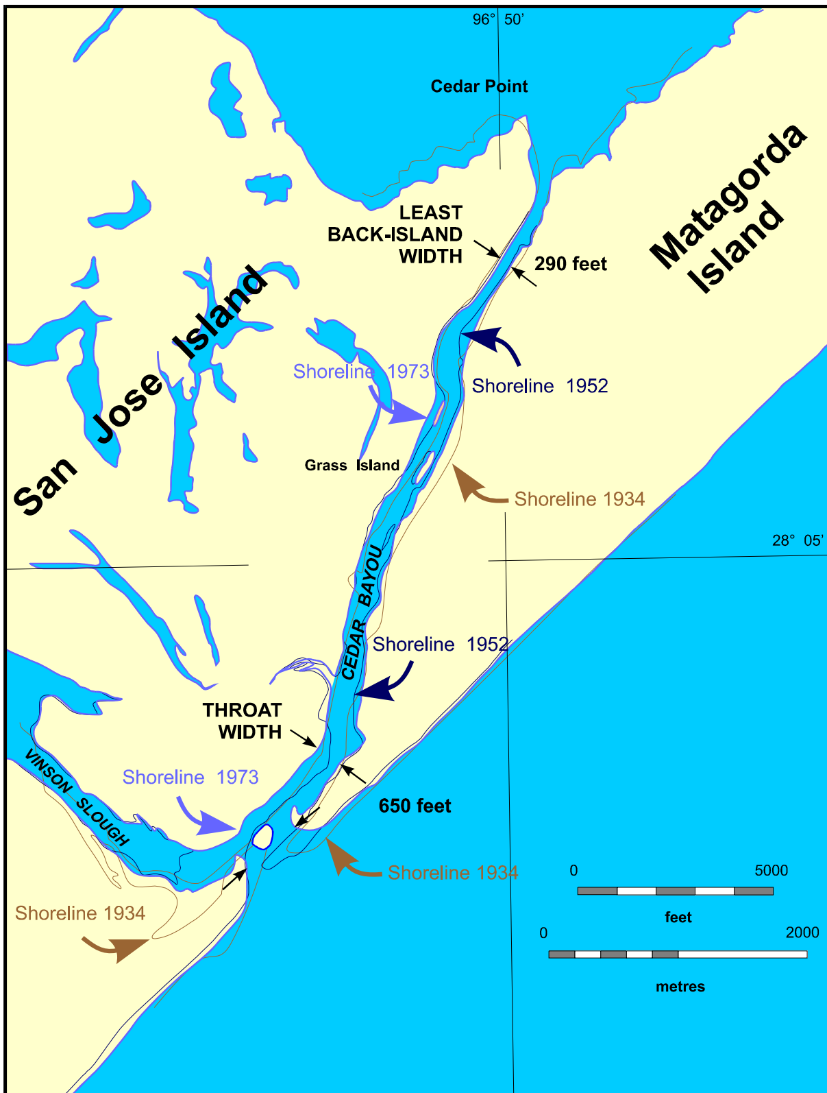
Figure 6 - Detail of Cedar Bayou showing three shorelines from the twentieth century, see text. The least back-island width and the throat width are based on the 1973 shoreline.
