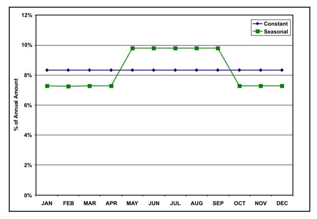
Figure 5-7. Model Simulated Constant Versus Seasonal Monthly Delivery Pattern from Lake Texana
