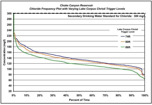
Figure 5-1. Impacts of Chloride Levels at CCR by Varying LCC Trigger Levels (Scenario 1)
