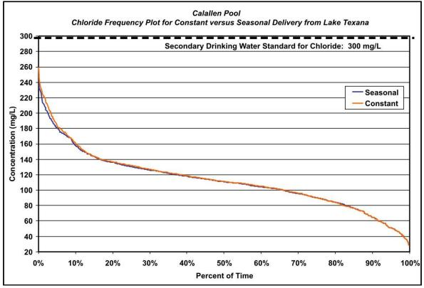
Figure 5-8. Impacts of Chloride Levels at Calallen Pool With Constant versus Season Delivery Patterns from Lake Texana (Scenario 3)
