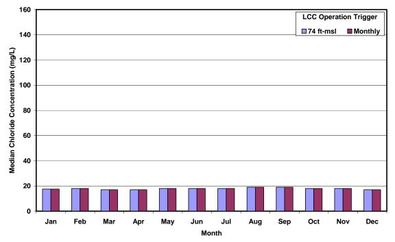
Lake Texana Chloride Frequency Plot for Constant versus Monthly Variable LCC triggers
