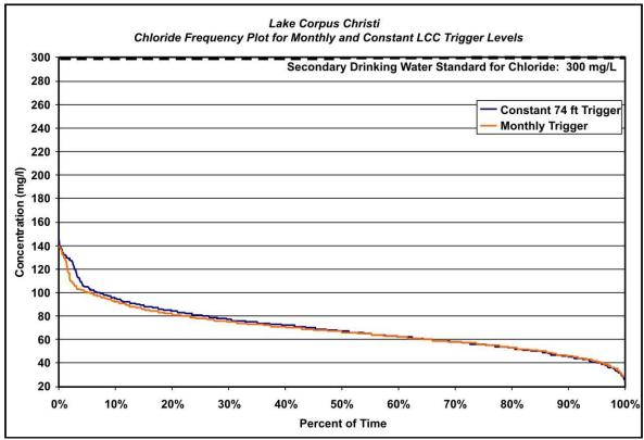
Figure 5-11. Impacts of Chloride Levels at LCC With Monthly Variable LCC Trigger Levels (Scenario 4)
