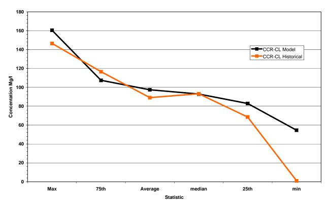
Calibrated Model Results: CCR Long Term Model Statistics for Chlorides
