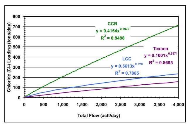
Figure 3-3. Chloride Loading of Inflows into CCR, LCC, and Lake Texana
