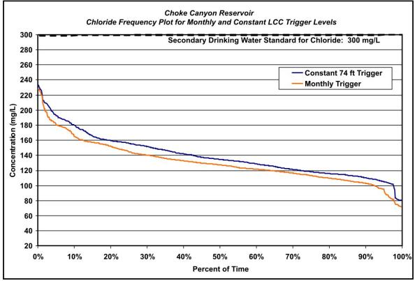
Figure 5-10. Impacts of Chloride Levels at CCR With Monthly Variable LCC Trigger Levels (Scenario 4)
