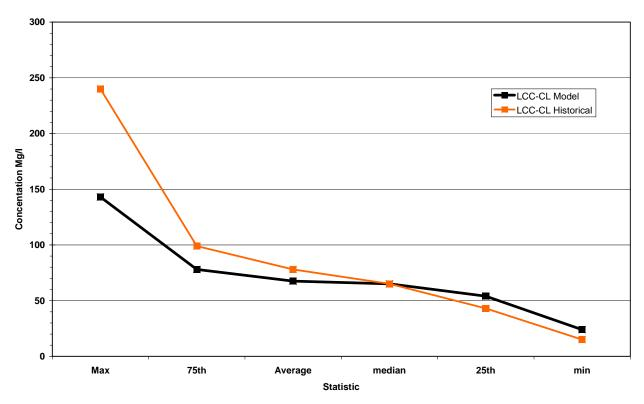
Calibrated Model Results: LCC Long Term Model Statistics for Chlorides
