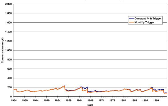
Choke Canyon Reservoir Chlorides Time Series for Monthly and 74ft Constant Trigger Levels
