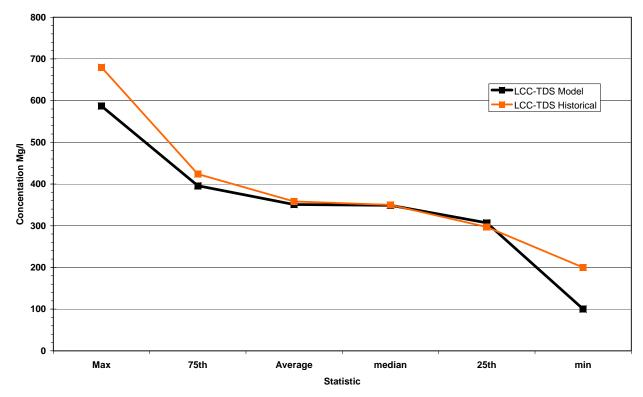
Calibrated Model Results: LCC Long Term Model Statistics for Total Dissolved Solids
