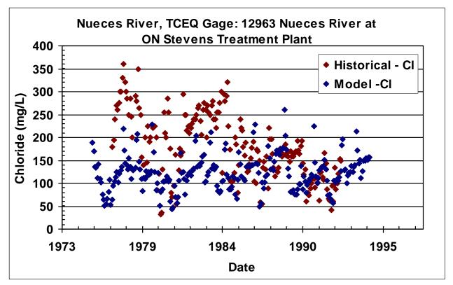
**Comparison of Historical Chloride Measurements to Calibrated Model Simulated Values**
