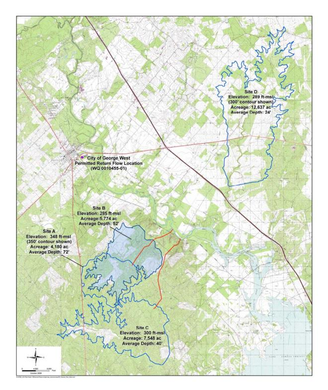
Figure 3-2. Alternative Reservoir Sites Considered for OCR (NOTE: Reservoir footprints based on 300,000 acft OCR)
