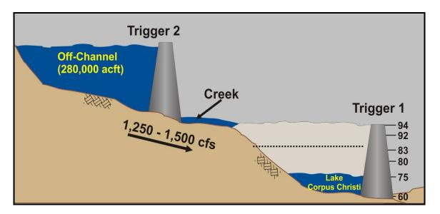
Figure 4-9. Recommended Pipeline Operations from OCR Storage to LCC
