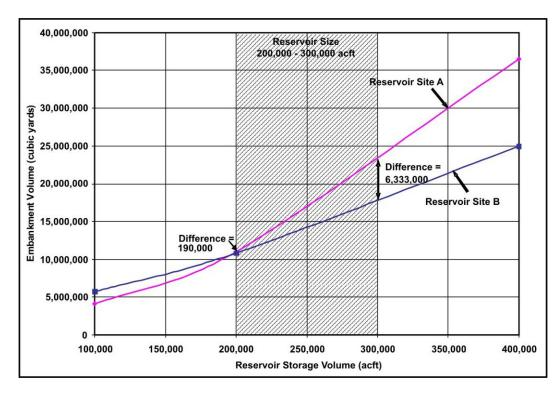
Figure 4-2. Comparison of Embankment Volumes for Reservoir Site A and B
