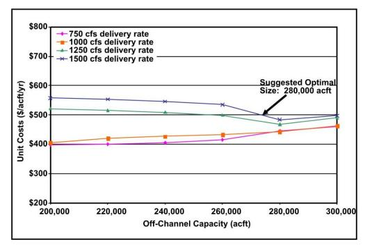
Figure 4-6. Unit Costs of Raw Water for Off-Channel Sizes (in Second Quarter 2007 Dollars)
