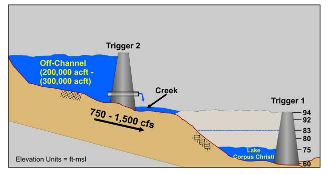
Figure 3-1. Pipeline Operations between LCC and OCR
