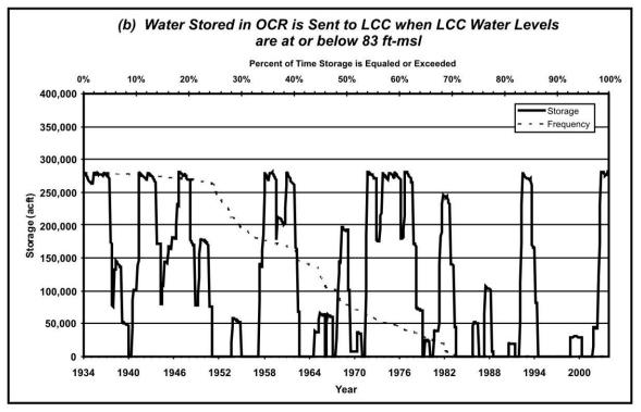
Figure 4-11. Storage and Frequency Plot of Operating OCR (280,000 acft Capacity at 1,500 cfs Pipeline Rate)
