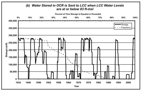
Figure 4-10. Storage and Frequency Plot of Operating OCR (280,000 acft Capacity at 1,250 cfs Pipeline Rate)
