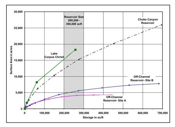
Figure 4-1. Comparison of Surface Area Required for Reservoir Sites A and B (as Compared to Lake Corpus Christi and Choke Canyon Reservoir)
