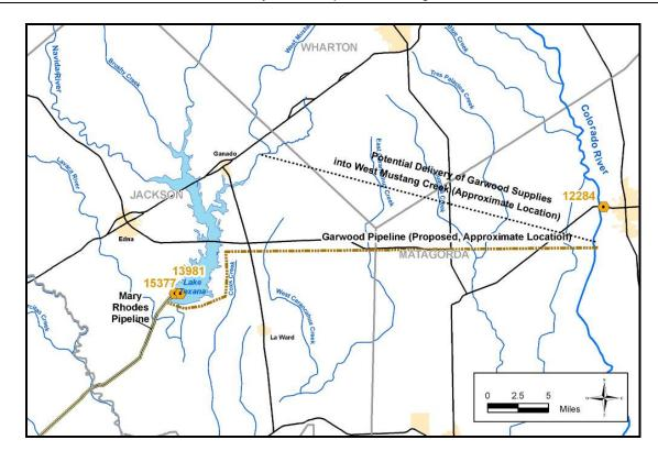
Figure 3-2. Water Quality Sampling Locations Used to Estimate Water Quality Data for the Garwood Project and Additional Lake Texana Supplies
