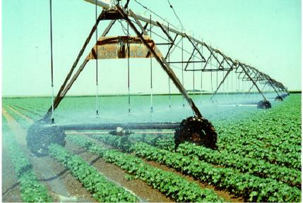
Figure 4: Photograph of center pivot technology
