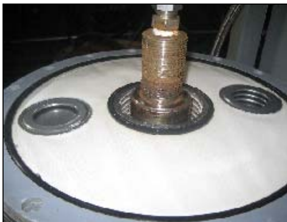
Figure 14: Top Membrane Tray at End of Testing
