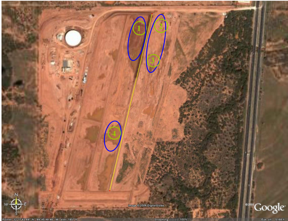
Note: Yellow line along the ponds is ~732 m (2,402 ft) long; blue outline shows water body at time of sampling; when picture was taken, the site was still apparently under construction Figure 12-11. Aerial view of evaporation pond of City of Abilene desalination facility showing sampling location (courtesy of Google Earth)
