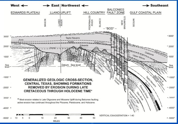
Generalized geologic cross-section, Central Texas, at present time, showing formations removed by Late Cretaceous through recent erosion; datum = modern sea-level; shaded area shows geologic section removed by post-Eocene erosion. Figure 29 from Rose, 2016.
