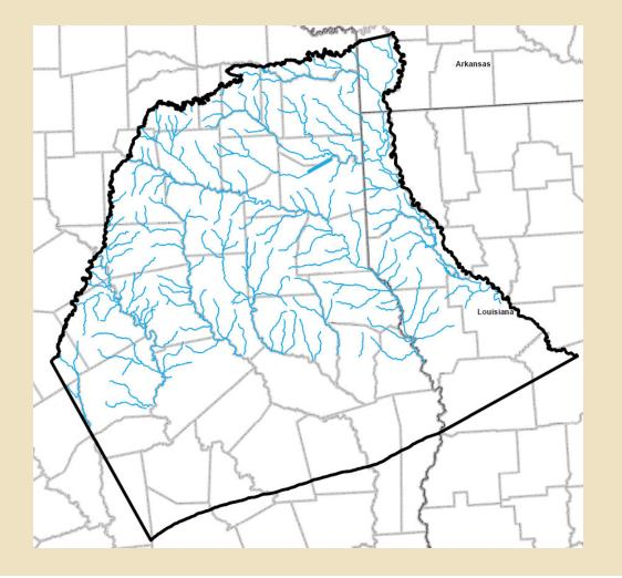
Stream network was generated based on the lowest elevations in the model domain based on the available DEM.
