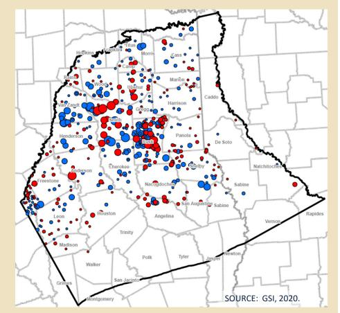
Figure Showing Average Error at Monitoring Wells from 1980 to 2013 (red: negative value; blue: positive value).
