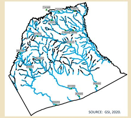
Simulated Rivers Showing Gaining Conditions (blue), Consistent with Measured Conditions.
