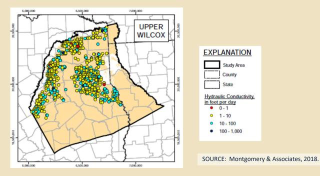
Example of Measured Hydraulic Conductivity Values Within Aquifer Units
