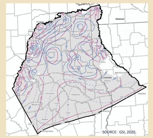
Example Flow Field for Middle Wilcox Aquifer (Layer 8), showing Simulated (purple) and Measured (blue) for 2013.
