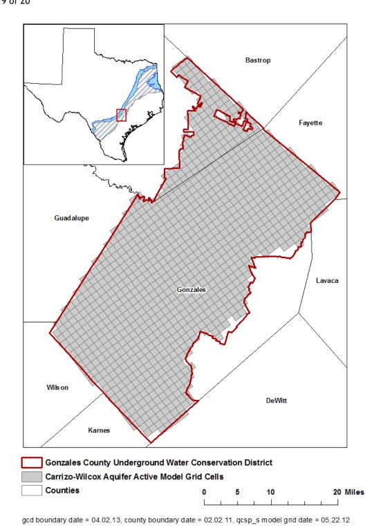
FIGURE 1: AREA OF THE GROUNDWATER AVAILABILITY MODEL FOR THE CARRIZO-WILCOX, QUEEN CITY, AND SPARTA AQUIFERS FROM WHICH THE INFORMATION FOR THE CARRIZO-WILCOX AQUIFER WAS EXTRACTED.
