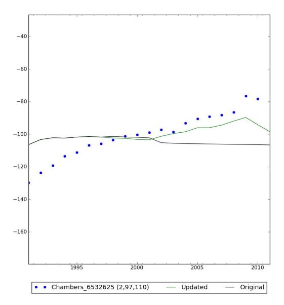
Figure A-2. Example hydrograph comparing the original and updated simulated water levels to measured water levels for the interim period in Chambers County.
