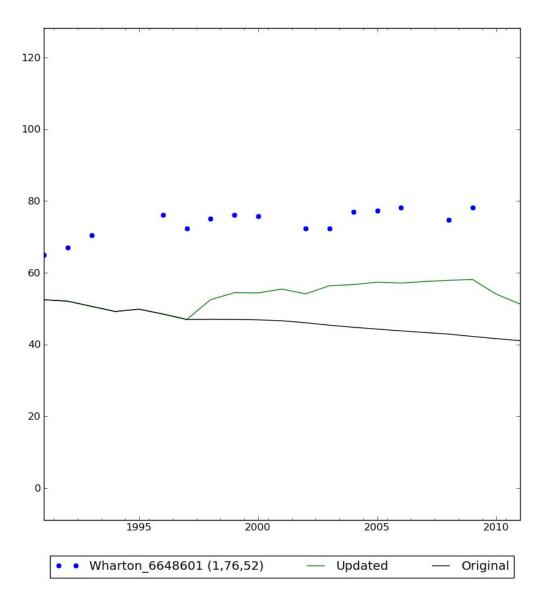
Figure A-8. Example hydrograph comparing the original and updated simulated water levels to measured water levels for the interim period in Wharton County.
