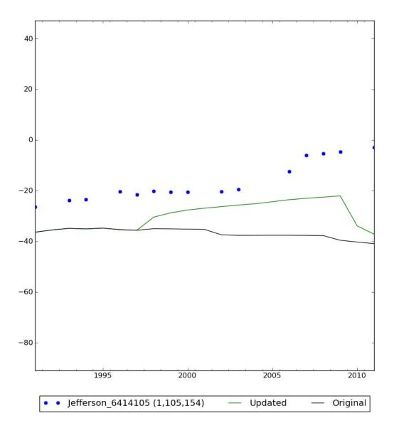
Figure A-3. Example hydrograph comparing the original and updated simulated water levels to measured water levels for the interim period in Jefferson County.
