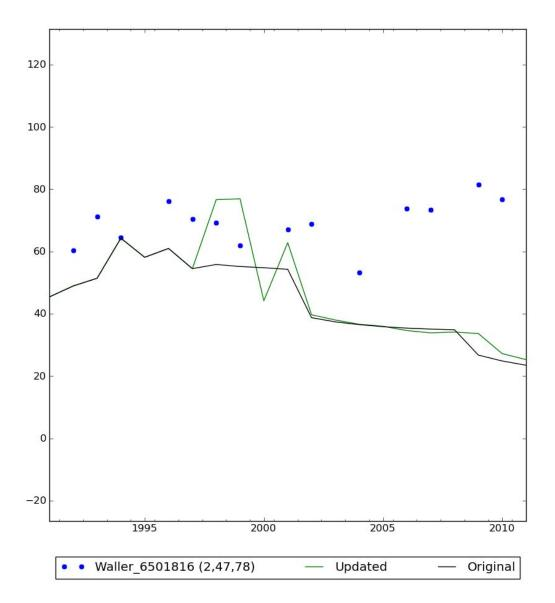
Figure A-7. Example hydrograph comparing the original and updated simulated water levels to measured water levels for the interim period in Waller County.
