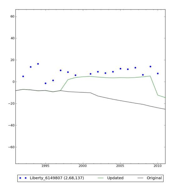
Figure A-4. Example hydrograph comparing the original and updated simulated water levels to measured water levels for the interim period in Liberty County.
