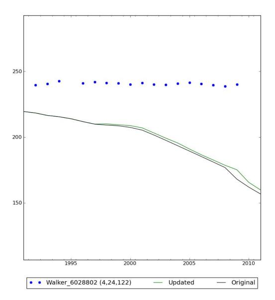
Figure A-6. Example hydrograph comparing the original and updated simulated water levels to measured water levels for the interim period in Walker County.
