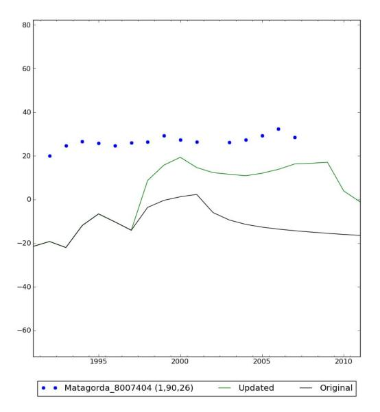
Figure A-5. Example hydrograph comparing the original and updated simulated water levels to measured water levels for the interim period in Matagorda County.
