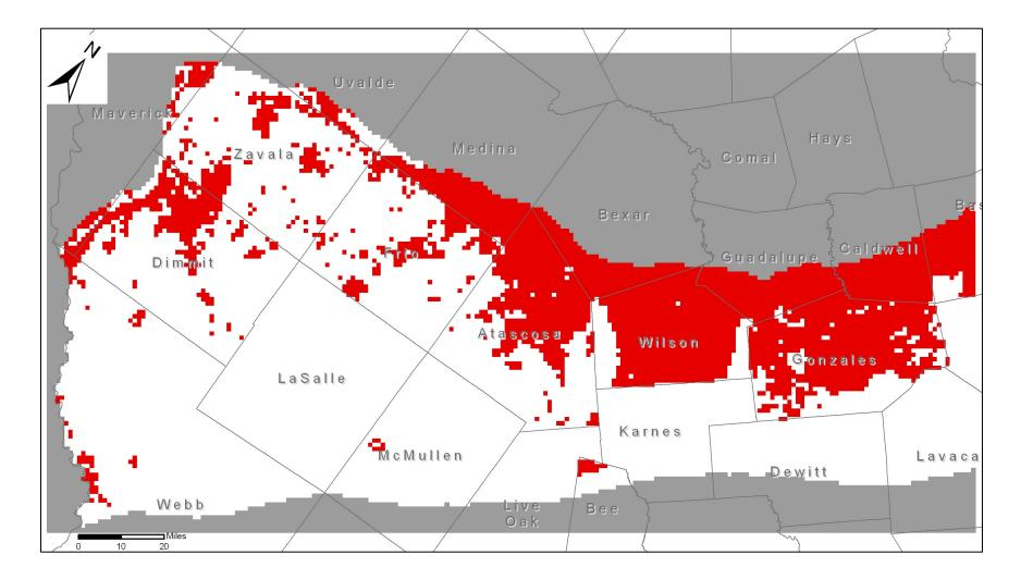
Figure A-22- Location of pumpage included in the groundwater availability model in the Middle Wilcox Aquifer (layer 7). Pumpage cells are in red. Active cells in this layer are in white.
