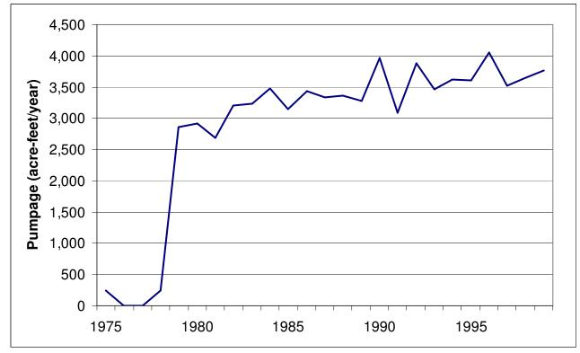
Figure A-4- Total pumpage in Caldwell County included in the groundwater availability model for the southern part of the Queen City-Sparta Aquifer.
