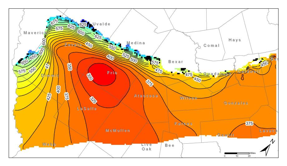
Figure 14. Water level elevations after 60 years using 1999 pumpage in the Lower Wilcox Aquifer. Water level elevations are in feet above mean sea level. Contour interval is 25 feet. Dry model cells are shown in black.
