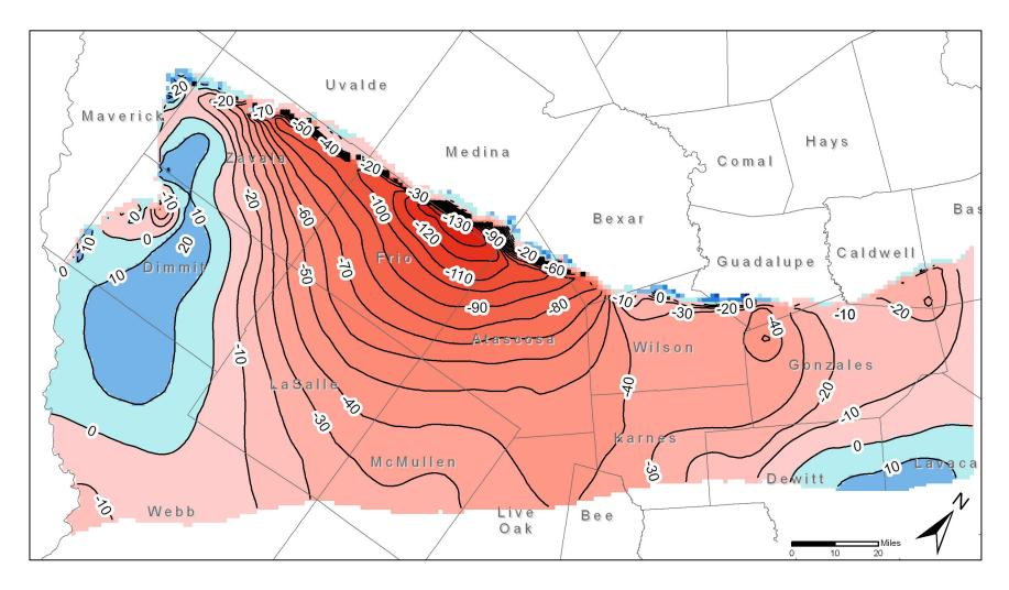
Figure 18. Water level changes after 60 years using 1999 pumpage in the Upper Wilcox Aquifer. Water level changes re in feet. Contour interval is 10 feet. Areas of increasing water levels are shown in blue. Areas of decreasing water levels are shown in red. Dry model cells are shown in black.
