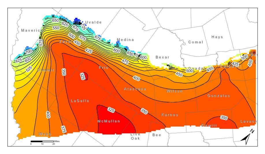
Figure 8. Initial water level elevations for the predictive model run in the Lower Wilcox Aquifer from the southern part of the Queen City, Sparta, and Carrizo-Wilcox aquifers groundwater availability model. Water level elevations are in feet above mean sea level. Contour interval is 25 feet.
