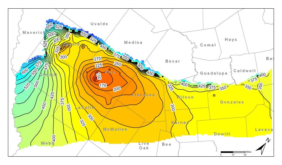
Figure 12. Water level elevations after 60 years using 1999 pumpage in the Upper Wilcox Aquifer. Water level elevations are in feet above mean sea level. Contour interval is 25 feet. Dry model cells are shown in black.
