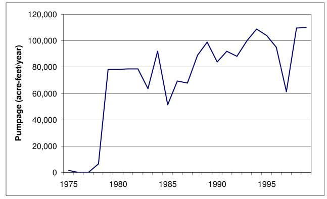
Figure A-6- Total pumpage in Frio County included in the groundwater availability model for the southern part of the Queen City-Sparta Aquifer.
