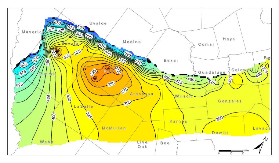
Figure 13. Water level elevations after 60 years using 1999 pumpage in the Middle Wilcox Aquifer. Water level elevations are in feet above mean sea level. Contour interval is 25 feet. Dry model cells are shown in black.
