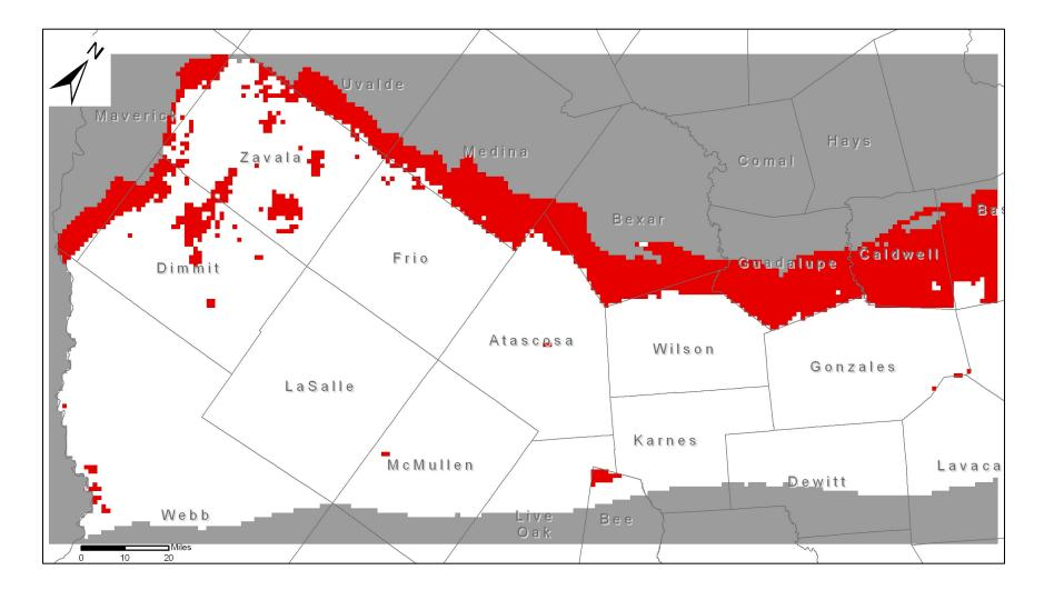
Figure A-23- Location of pumpage included in the groundwater availability model in the Lower Wilcox Aquifer (layer 8). Pumpage cells are in red. Active cells in this layer are in white.
