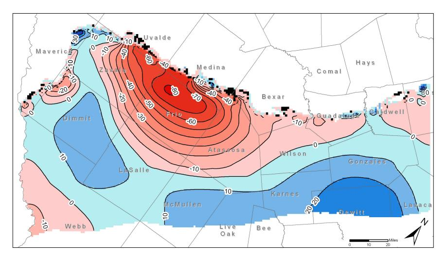
Figure 20. Water level changes after 60 years using 1999 pumpage in the Lower Wilcox Aquifer. Water level changes are in feet. Contour interval is 10 feet. Areas of increasing water levels are shown in blue. Areas of decreasing water levels are shown in red. Dry model cells are shown in black.
