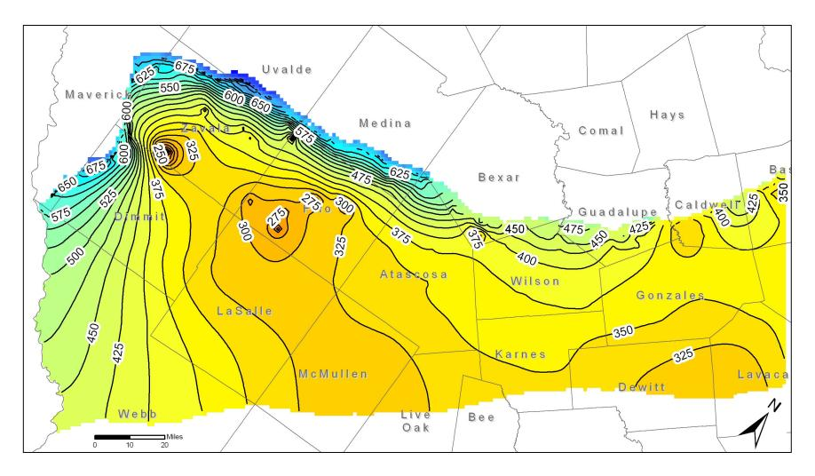
Figure 7. Initial water level elevations for the predictive model run in the Middle Wilcox Aquifer from the southern part of the Queen City, Sparta, and Carrizo-Wilcox aquifers groundwater availability model. Water level elevations are in feet above mean sea level. Contour interval is 25 feet.
