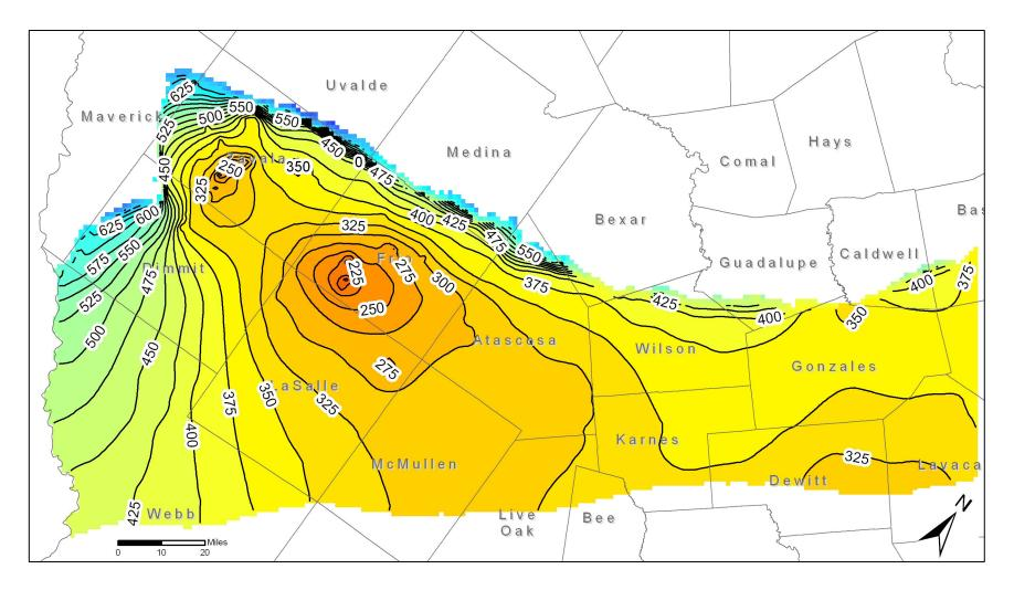
Figure 6. Initial water level elevations for the predictive model run in the Upper Wilcox Aquifer from the southern part of the Queen City, Sparta, and Carrizo-Wilcox aquifers groundwater availability model. Water level elevations are in feet above mean sea level. Contour interval is 25 feet.
