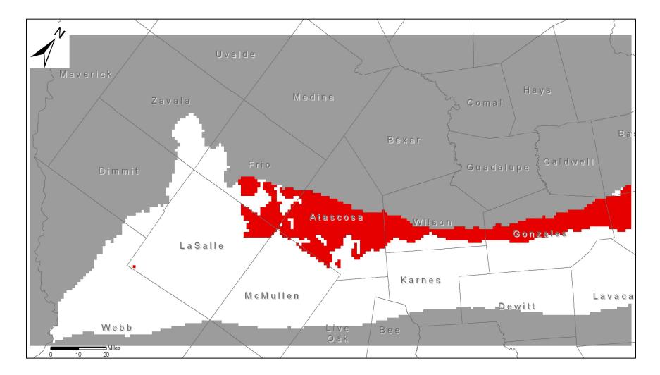
Figure A-18- Location of pumpage included in the groundwater availability model in the Sparta Aquifer (layer 1). Pumpage cells are in red. Active cells in this layer are in white.
