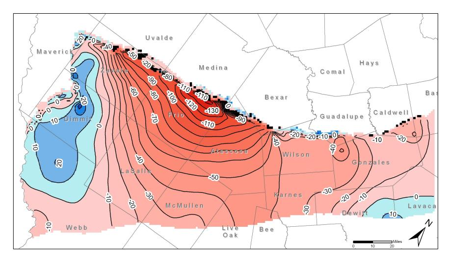
Figure 17. Water level changes after 60 years using 1999 pumpage in the Carrizo Aquifer. Water level changes are in feet. Contour interval is 10 feet. Areas of increasing water levels are shown in blue. Areas of decreasing water levels are shown in red. Dry model cells are shown in black.
