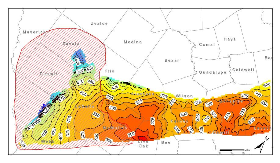
Figure 9. Water level elevations after 60 years using 1999 pumpage in the Sparta Aquifer. Water level elevations are in feet above mean sea level. Contour interval is 25 feet. Dry model cells are shown in black. The area west of the Frio River (shown in red) is not considered to be part of the Sparta Aquifer and does not have any pumpage assigned to it.
