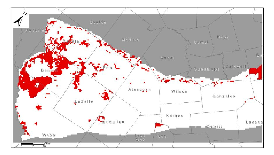
Figure A-21- Location of pumpage included in the groundwater availability model in the Upper Wilcox Aquifer (layer 6). Pumpage cells are in red. Active cells in this layer are in white.
