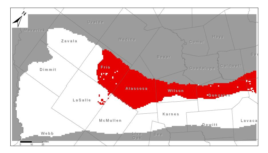
Figure A-19- Location of pumpage included in the groundwater availability model in the Queen City Aquifer (layer 3). Pumpage cells are in red. Active cells in this layer are in white.
