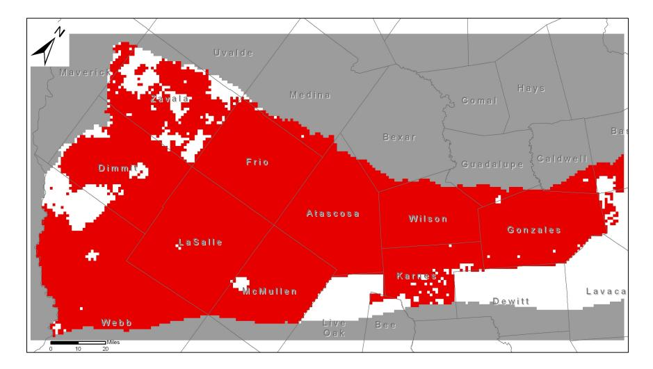
Figure A-20- Location of pumpage included in the groundwater availability model in the Carrizo Aquifer (layer 5). Pumpage cells are in red. Active cells in this layer are in white.
