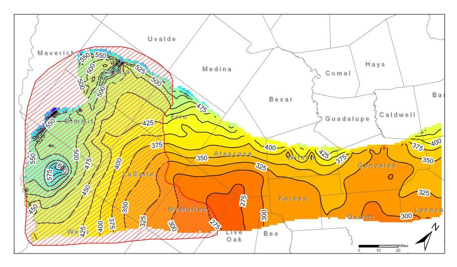
Figure 10. Water level elevations after 60 years using 1999 pumpage in the Queen City Aquifer. Water level elevations are in feet above mean sea level. Contour interval is 25 feet. Dry model cells are shown in black. The area west of the Frio River (shown in red) is not considered to be part of the Queen City Aquifer and does not have any pumpage assigned to it.
