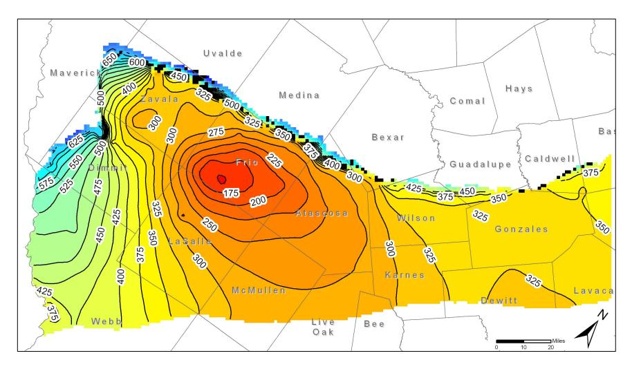
Figure 11. Water level elevations after 60 years using 1999 pumpage in the Carrizo Aquifer. Water level elevations are in feet above mean sea level. Contour interval is 25 feet. Dry model cells are shown in black.
