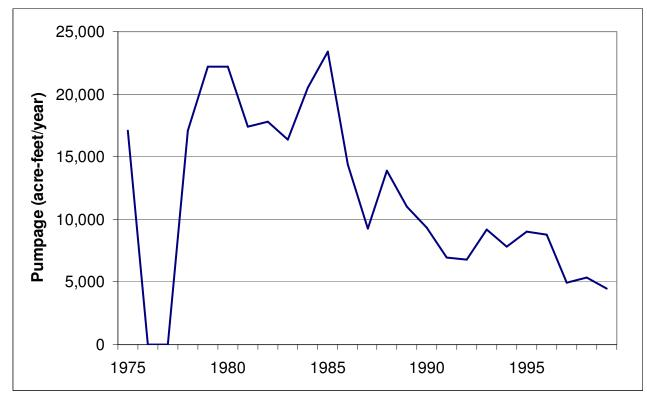
Figure A-5- Total pumpage in Dimmit County included in the groundwater availability model for the southern part of the Queen City-Sparta Aquifer.
