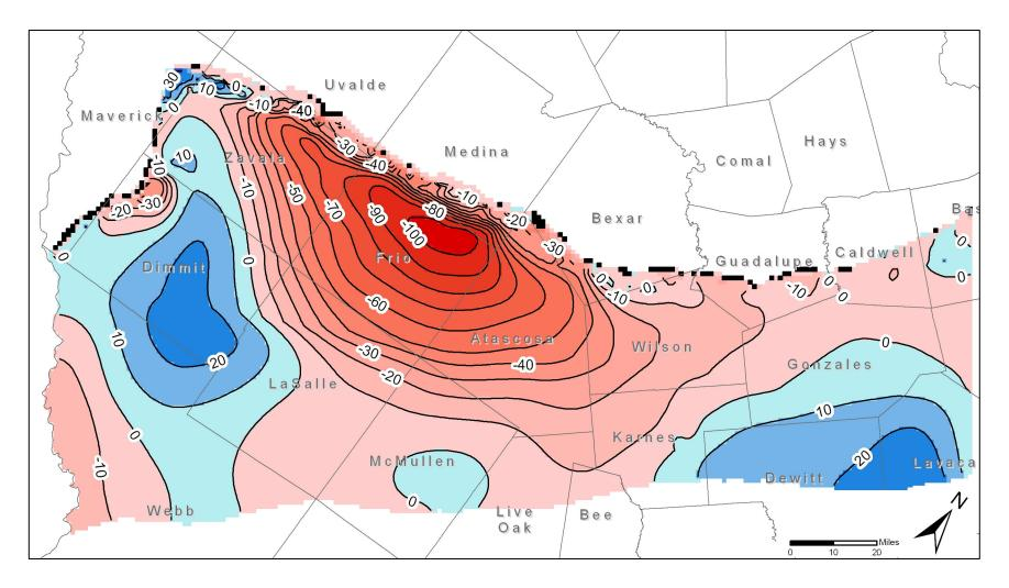
Figure 19. Water level changes after 60 years using 1999 pumpage in the Middle Wilcox Aquifer. Water level changes are in feet. Contour interval is 10 feet. Areas of increasing water levels are shown in blue. Areas of decreasing water levels are shown in red. Dry model cells are shown in black.
