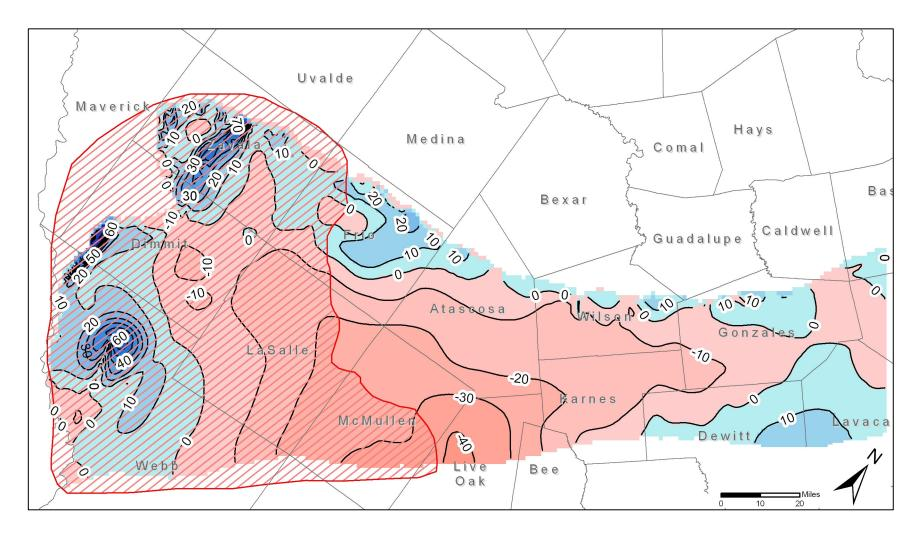
Figure 16. Water level changes after 60 years using 1999 pumpage in the Queen City Aquifer. Water level changes are in feet. Contour interval is 10 feet. Areas of increasing water levels are shown in blue. Areas of decreasing water levels are shown in red. Dry model cells are shown in black. The area west of the Frio River (shown in red) is not considered to be part of the Queen City Aquifer and does not have any pumpage assigned to it.
