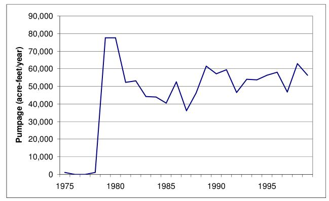
Figure A-1- Total pumpage in Atascosa County included in the groundwater availability model for the southern part of the Queen City-Sparta Aquifer.
