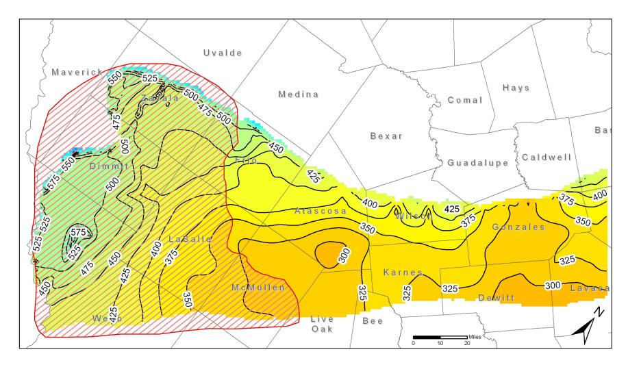
Figure 4. Initial water level elevations for the predictive model run in the Queen City Aquifer from the southern part of the Queen City, Sparta, and Carrizo-Wilcox aquifers groundwater availability model. Water level elevations are in feet above mean sea level. Contour interval is 25 feet. The area west of the Frio River (shown in red) is not considered to be part of the Queen City Aquifer and does not have any pumpage assigned to it.
