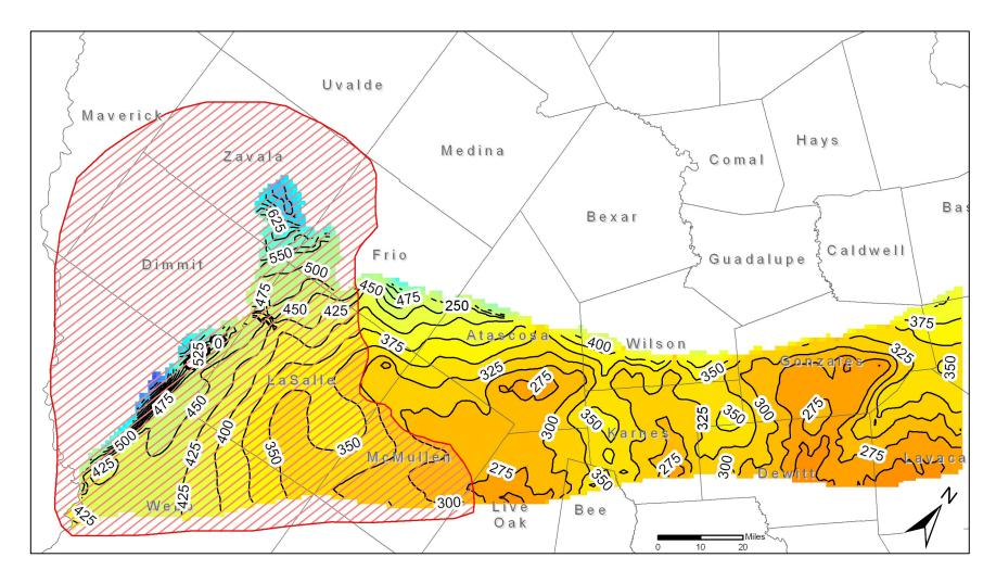
Figure 3. Initial water level elevations for the predictive model run in the Sparta Aquifer from the southern part of the Queen City, Sparta, and Carrizo-Wilcox aquifers groundwater availability model. Water level elevations are in feet above mean sea level. Contour interval is 25 feet. The area west of the Frio River (shown in red) is not considered to be part of the Sparta Aquifer and does not have any pumpage assigned to it.
