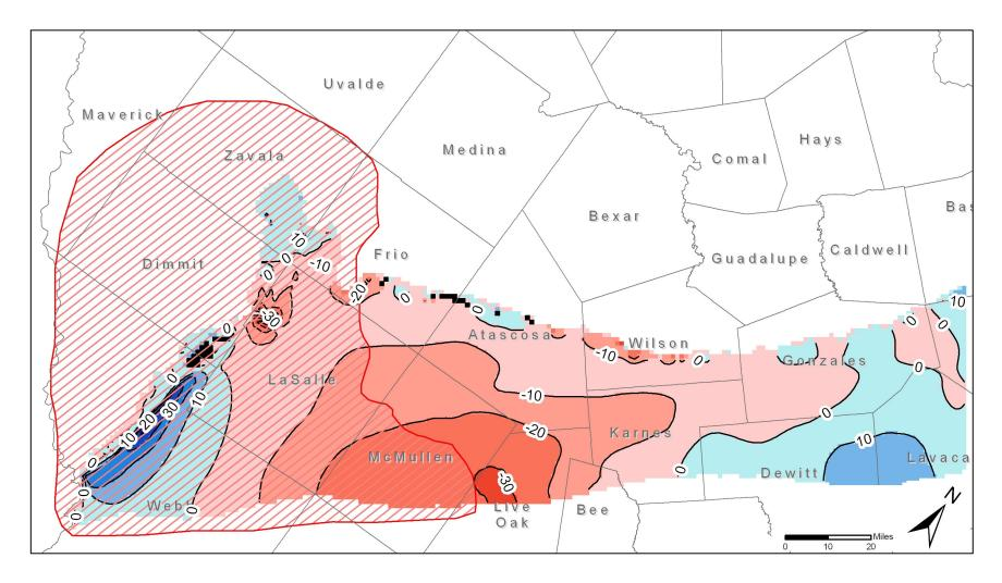
Figure 15. Water level changes after 60 years using 1999 pumpage in the Sparta Aquifer. Water level changes are in feet. Contour interval is 10 feet. Areas of increasing water levels are shown in blue. Areas of decreasing water levels are shown in red. Dry model cells are shown in black. The area west of the Frio River (shown in red) is not considered to be part of the Sparta Aquifer and does not have any pumpage assigned to it.
