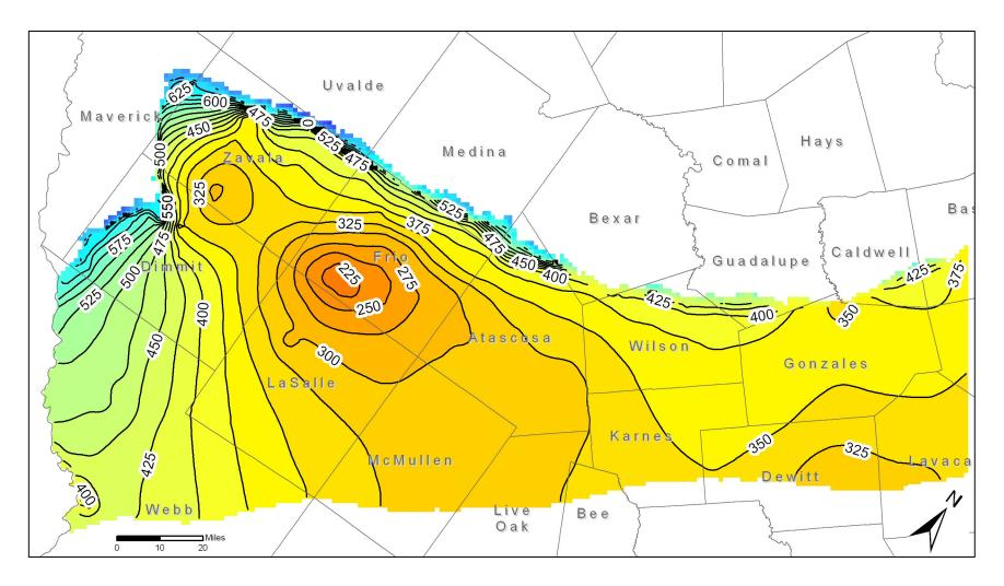
Figure 5. Initial water level elevations for the predictive model run in the Carrizo Aquifer from the southern part of the Queen City, Sparta, and Carrizo-Wilcox aquifers groundwater availability model. Water level elevations are in feet above mean sea level. Contour interval is 25 feet.
