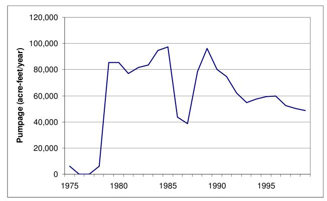
Figure A-17- Total pumpage in Zavala County included in the groundwater availability model for the southern part of the Queen City-Sparta Aquifer.
