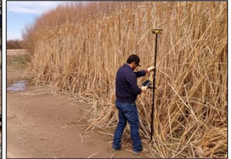
Vegetated Sandbar Limiting Flow Capacity in the Rio Grande Image: "Evaluation of Reduced Flow Capacity of the Rio Grande and the Impacts on the Operations of the Rio Grande Project Leasburg Dam to American Dam" (Joint Committee on Rio Grande Project Flood Risk (2019))
