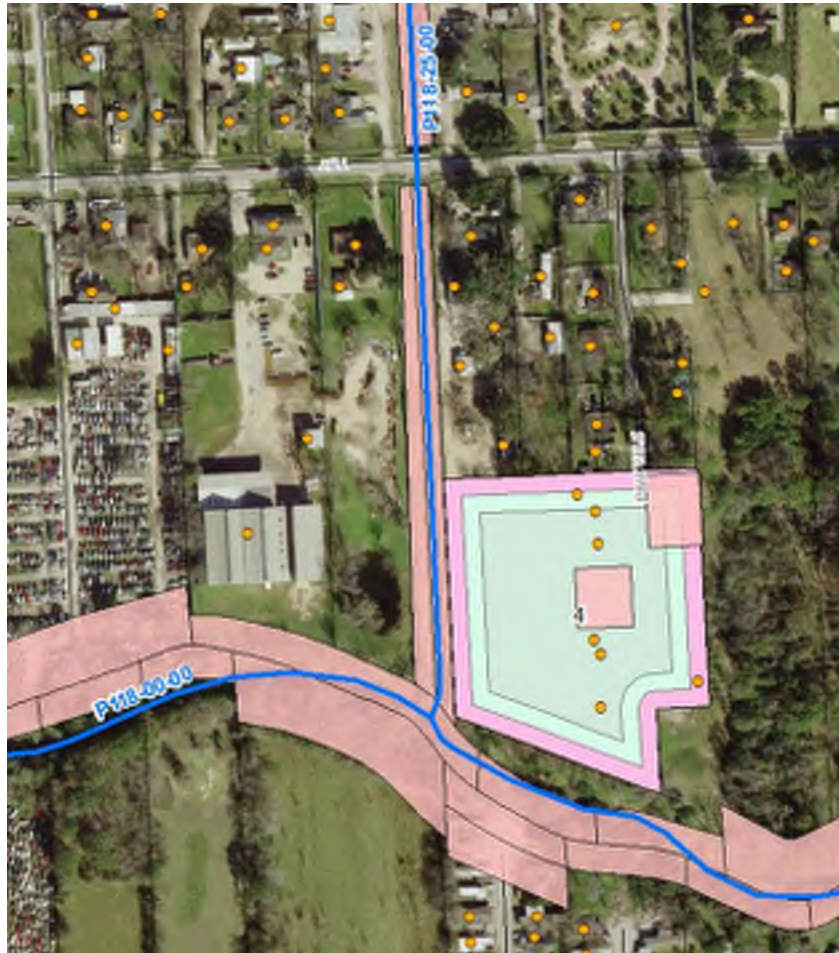
Figure 3-5: Feature 4 “Wooded Basin” – Layout and Location with Existing HCFCD ROW (red)
