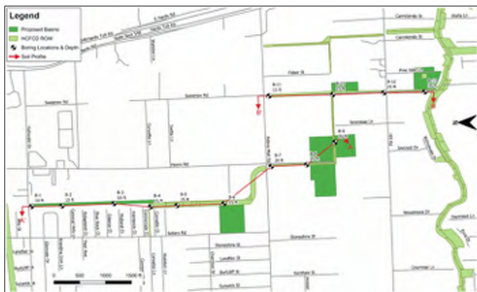
Figure 6-1: Soil Boring Locations
